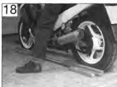
Two straightedges are used to check wheel alignment
