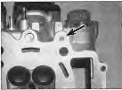
11.11 Blow compressed air through the oil nozzle (arrowed) to ensure it is clear
