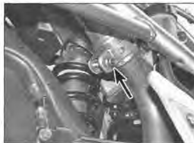
13.3 Slacken the clamp bolt (arrowed) between the mid-section and the silencer front pipe
