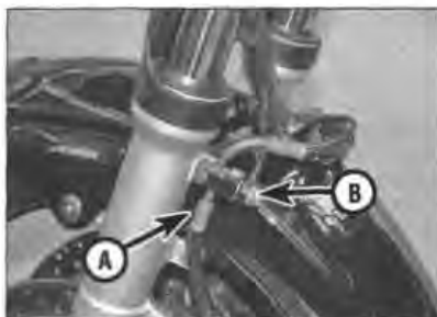
10.4d Front caliper link hose (A) and ABS hose banjo union (B)
