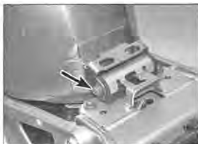
2.2 Loosen the bolt (arrowed) at the rear of the tank
