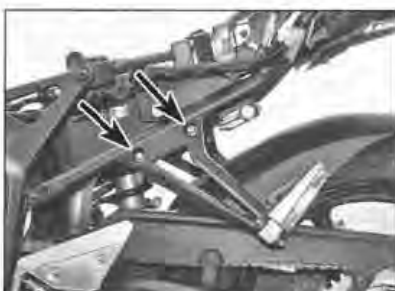
3.4b Passenger footrest brackets are bolted to the rear sub-frame (arrowed) – S2 models
