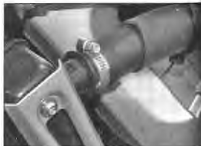
2.6b . . . and the radiator inlet hose from their unions
