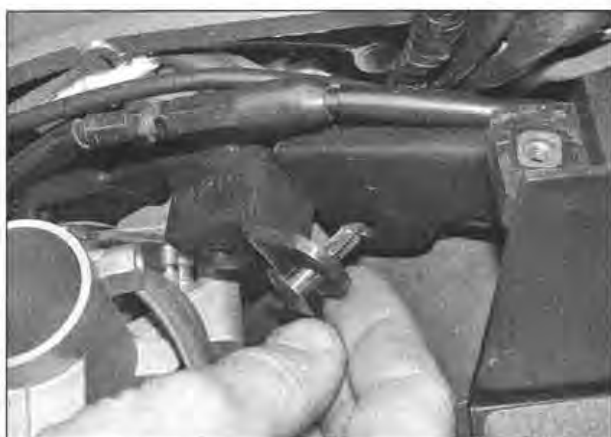
6.7c ... so that the clutch cable support bracket can be displaced
