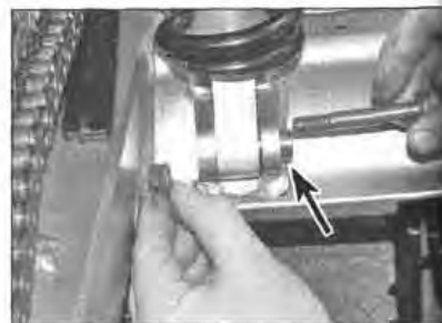
11.5a Remove the lower mounting bolt, noting the sleeve (arrowed)
