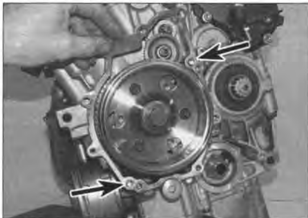
31.14 Ensure the cover gasket locates on the dowels (arrowed)
