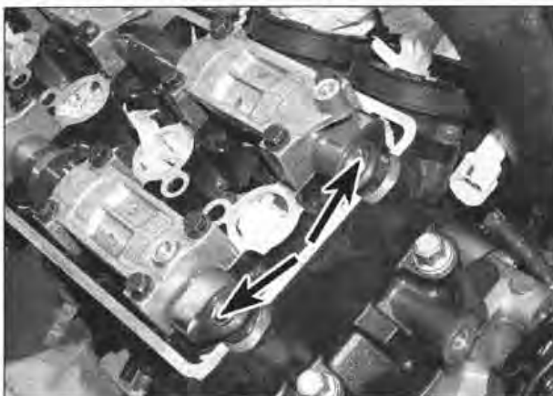
8.4c The camshaft lobes should face away from each other as shown
