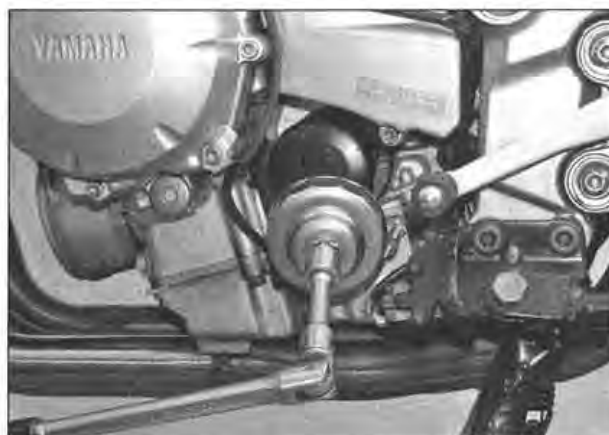
10.10 Ensure the filter removing tool is a good fit on the cartridge
