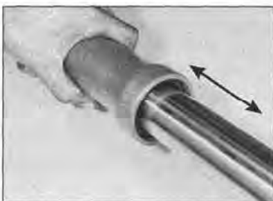
8.8a To separate the inner tube from the outer tube, pull them apart firmly several times . . .
