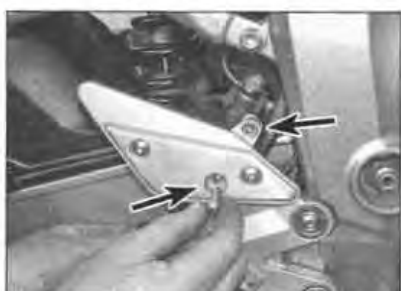
3.16 Rear brake master cylinder is secured by two bolts (arrowed)
