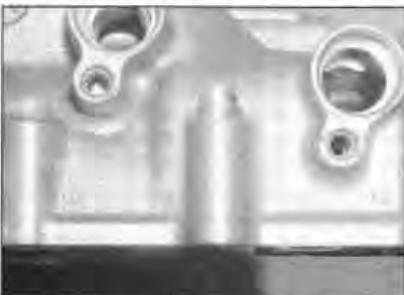
28.6b ... and blow through the oil passageways with compressed air
