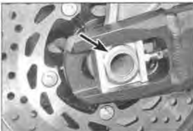
15.5b On S2 models, note how the axle (arrowed) locates inside the right-hand axle plate
