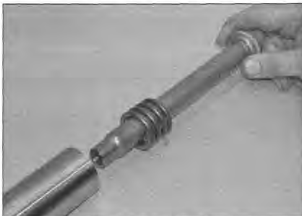
8.9 Withdraw the damper and spring
