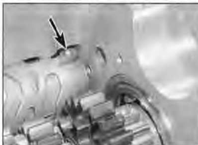
27.16b Neutral contact on the drum (arrowed) should align with the neutral switch
