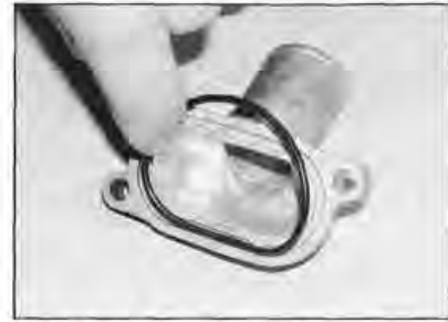
8.4c Note the location of the sealing O-ring
