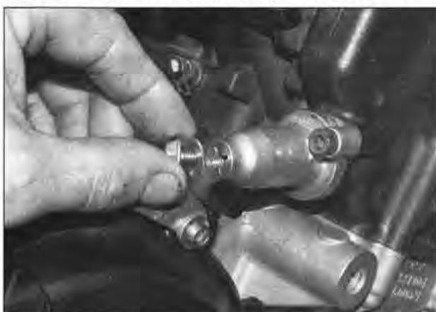
7.11 Fit the cap bolt using a new sealing washer
