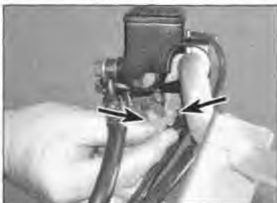
5.3 Front brake light switch wiring connectors (arrowed)
