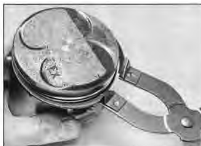
22.4a Removing the piston rings using a ring removal and installation tool
