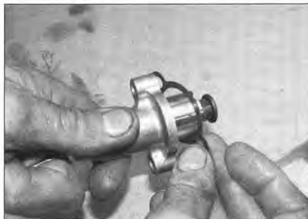
7.9 Fit a new gasket onto the tensioner . . .
