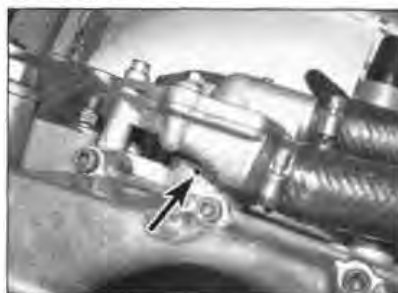
7.3 Water pump drain hole (arrowed)
