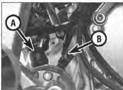
8.45 Location of the starter motor terminal (A) and speed sensor (B)
