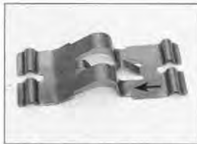
2.28 Arrow on pad spring should point to the front
