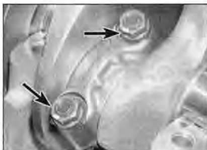
21.36c Alternatively, make reference marks (arrowed) with a dab of paint . . .
