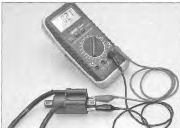
17.4 Checking the coil primary resistance between the wiring terminals
