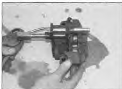
3.33c Holding the pistons with a retracting tool and brake pad
