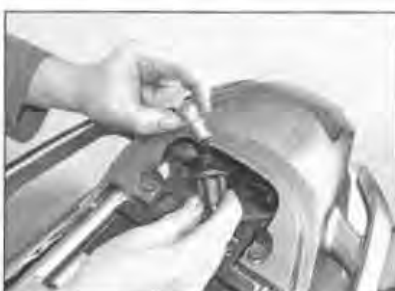
9.3 Push the bulb and twist it anti-clockwise to remove it
