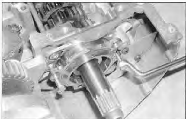
25.5b . . . and turning them against the crankcase surface
