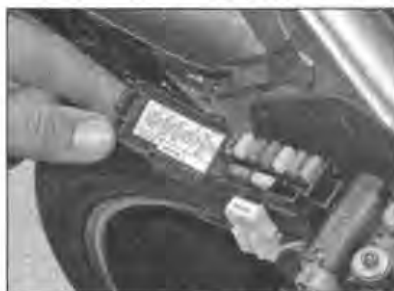
5.1b Location of the fusebox behind the right-hand side panel
