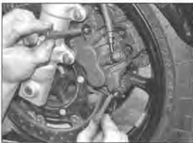
2.1a Undo the slider pins ...
