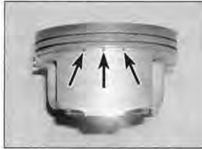
22.7a Ensure that the oil return holes (arrowed) are clear . . .
