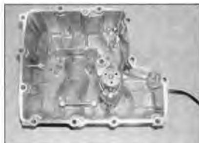
17.6 Clean the inside of the sump thoroughly
