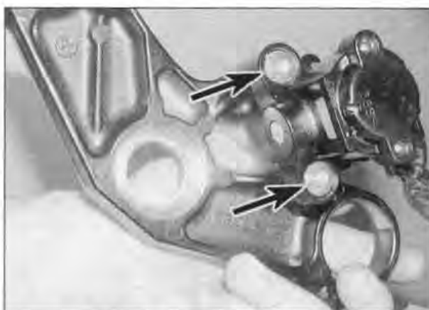
18.10 Remove the shear-head bolts (arrowed)
