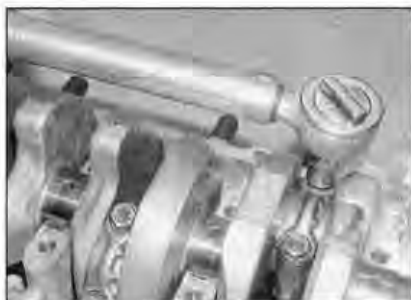
21.36a Tighten the nuts/bolts to the initial torque setting with a torque wrench . . .
