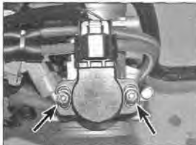
8.25 Throttle position sensor is secured by Torx screws (arrowed)
