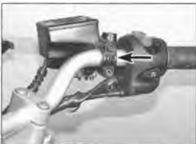
5.4b Unscrew the clamp bolts and remove clamp
