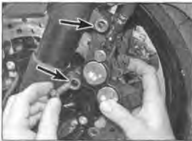
3.26b Unscrew the mounting bolts (arrowed) . . .
