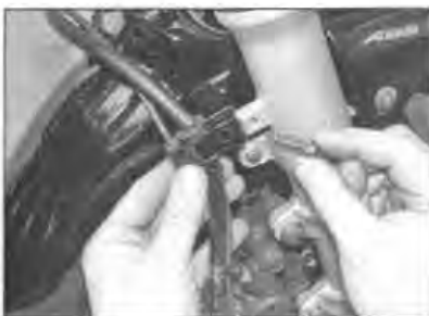
3.2a Unscrew the bolt securing the brake hose to the fork leg
