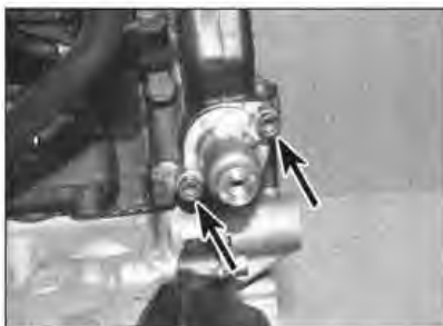
7.4a Slacken the mounting bolts (arrowed) slightly ...
