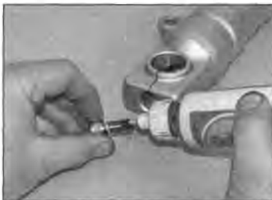
8.22b . . . and apply locking compound to the bolt threads
