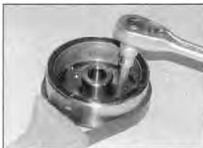
14.5b Remove the bolts to separate the starter clutch from the alternator rotor
