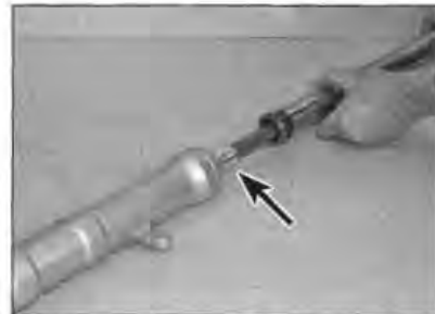
8.21 Installing the inner tube/damper assembly – note the damper seat (arrowed)
