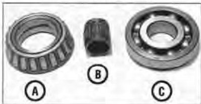
5.15 Tapered roller bearing (A), needle roller bearing (B) and ball journal bearing (C)
