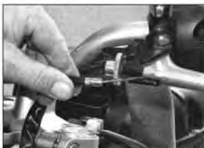
12.5b Align the slots in the adjuster and the bracket and pull the cable out
