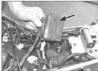
17.107b ... and displace the ABS control unit (arrowed)
