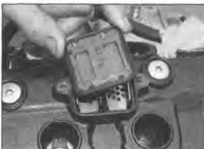
14.14b Lift out the reed valve ...
