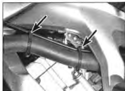
12.6 Clutch cable is secured to the coolant hose by ties (arrowed)
