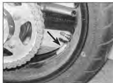
12.2b Check the security of any wheel balance weights (arrowed)
