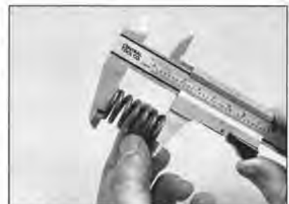
13.21 Measure the free length of the clutch springs as shown
