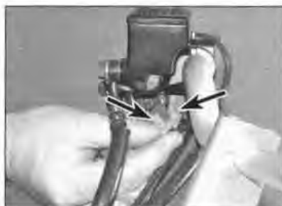
14.2 Front brake light switch wiring connectors (arrowed)
