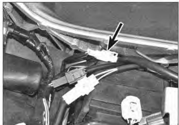
4.11e Disconnect the neutral switch wiring connector
