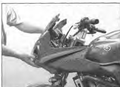
5.11 Draw the fairing off its support bracket
