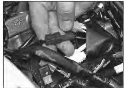
4.11c ... the sidestand switch wiring connector ...
