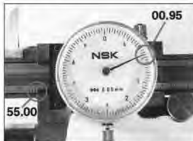
3.14 Vernier gauge reading of 55.95 mm
