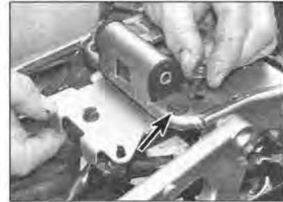
32.8b ... then install the mounting screws. Note the mounting bush (arrowed)
