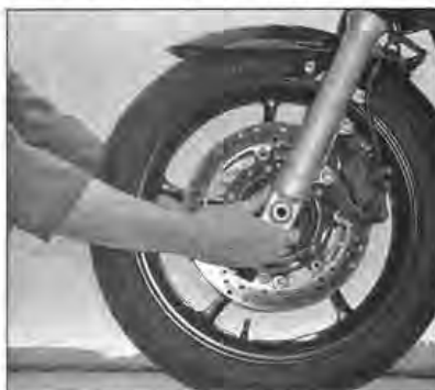
14.5 Checking for play in the steering head bearings
