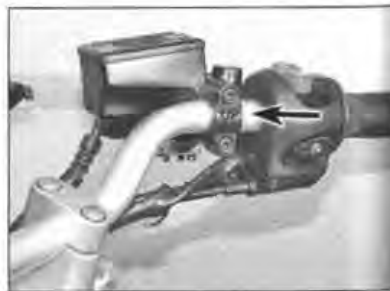
5.22 Note the UP mark (arrowed) on the clamp
