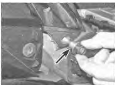
6.7 Note how the spacers (arrowed) fit on the side mounting bolts
