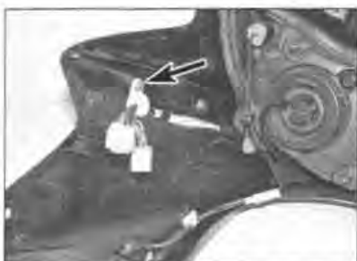
8.17 Headlight sub-loom wiring is secured by clip (arrowed)
