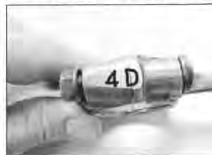
21.25b Connecting rod size code number
