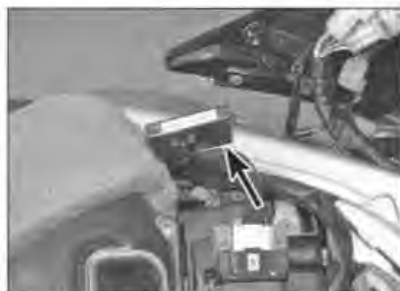
5.1d Fusebox (arrowed) houses the ABS control unit and modulator fuses
