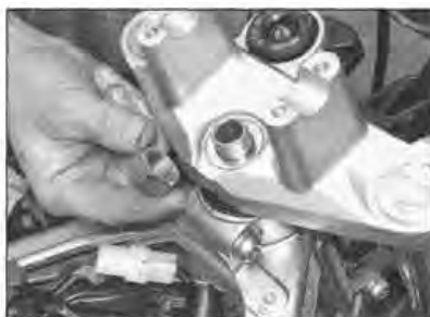
9.10a Undo the steering stem nut ...
