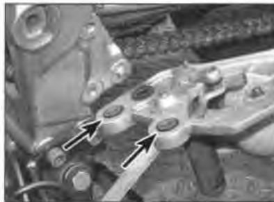
3.8b . . . and lift the assembly off. Note the collars and bushes (arrowed)
