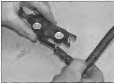
9.7 Disconnect the reservoir hose from the union on the master cylinder
