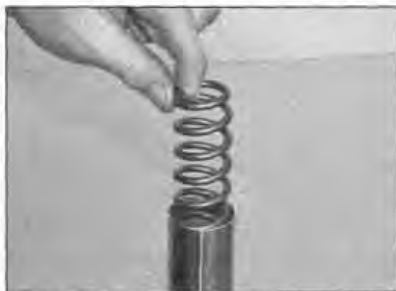
7.3c ... then pull out the spring
