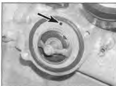
6.10 Install thermostat with breather hole (arrowed) at top
