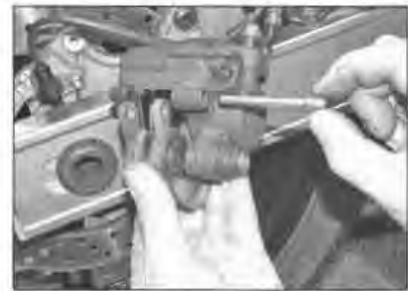
6.4b . . . then undo the pad pin and remove the pads
