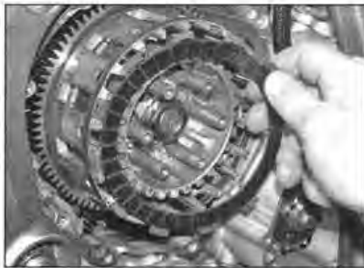
13.37b ... then a purple-coded friction plate ...
