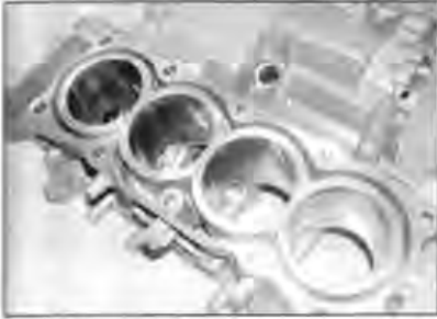
28.18 Examine the cylinder walls carefully
