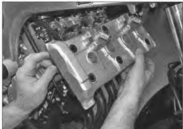
19.4 Valve cover can be lifted off towards the front
