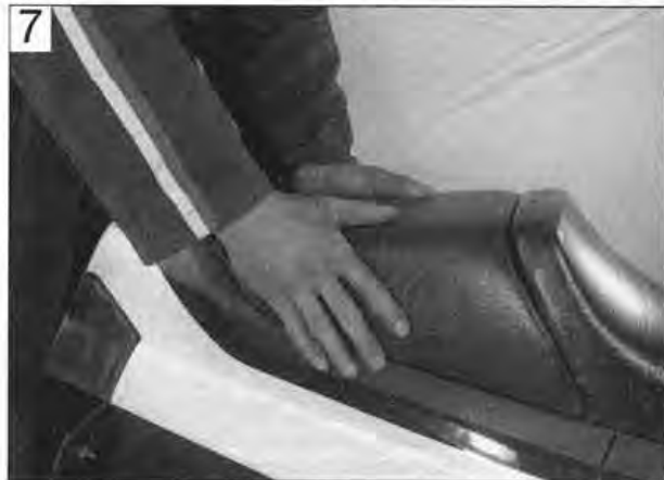
Bounce the rear of the motorcycle to check rear suspension operation
