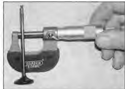
11.19 Measuring valve stem diameter with a micrometer
