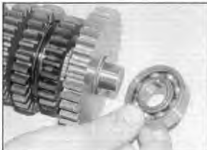
26.49 ... and fit the bearing
