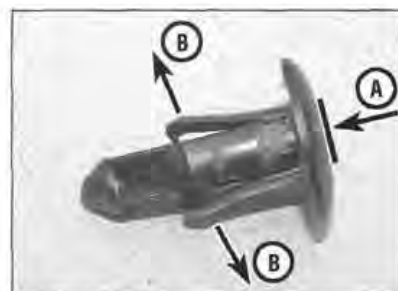
11.14b Push the centre (A) in to extend the locking tabs (B)
