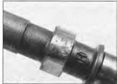
8.15a Check the camshaft lobes as described – damage as shown requires immediate attention
