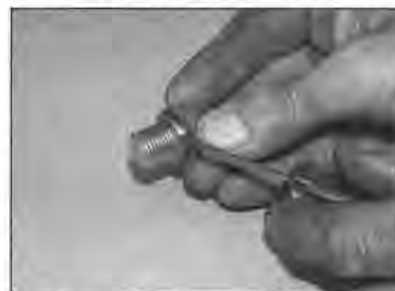
10.4b Replace the old sealing washer with a new one
