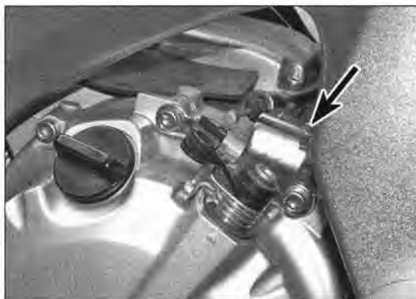
13.5b ... noting the location of the cable bracket (arrowed)
