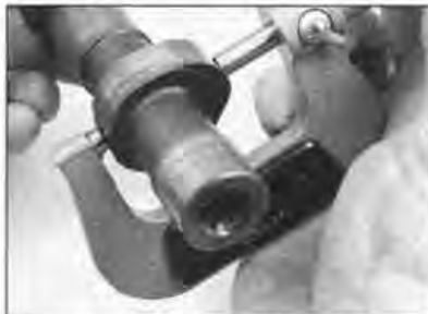
8.15b Measure the height of the camshaft lobes with a micrometer
