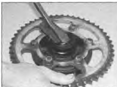
16.22 Lever the bearing seal out of the coupling
