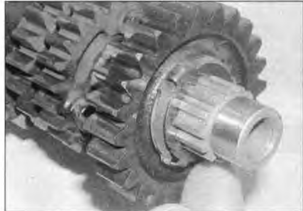
26.25 . . . then slide on the tabbed lockwasher . . .
