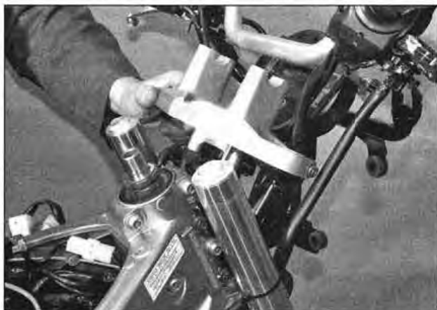
14.8c Ease the top yoke off
