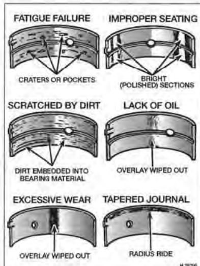
5.17 Typical bearing failures
