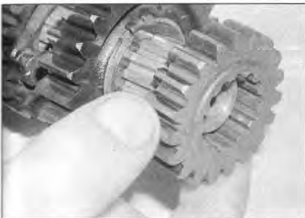
26.26 . . . and the 2nd gear pinion
