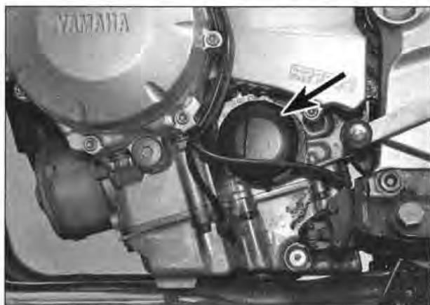
10.9 Location of the oil filter (arrowed)
