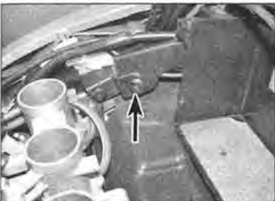
12.2a Press in the centre of the trim clip (arrowed) ...
