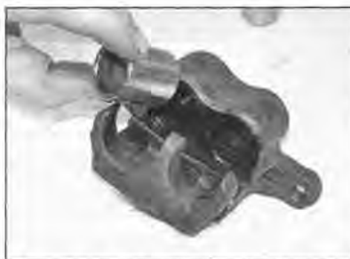
3.16a Install the pistons closed end first
