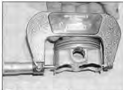
22.10 Measuring the piston diameter with a micrometer
