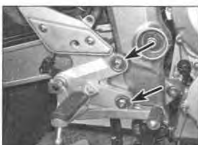
3.17a Unscrew the mounting bolts (arrowed) ...
