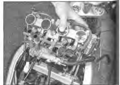
9.9 Ease the throttle body assembly off
