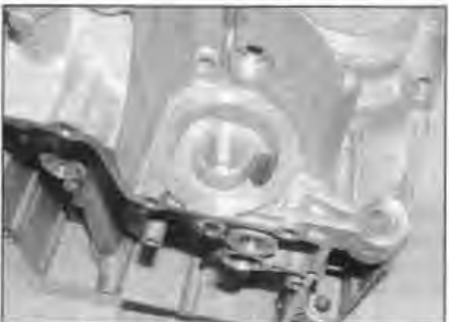
28.6a Clean the crankcases thoroughly ...
