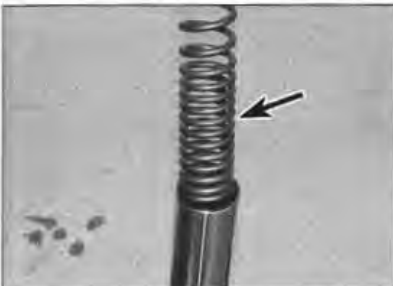
7.8 Closer-wound coils (arrowed) should be at the bottom of the spring
