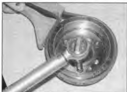
14.12 Apply locking compound to the starter clutch bolts and tighten them securely
