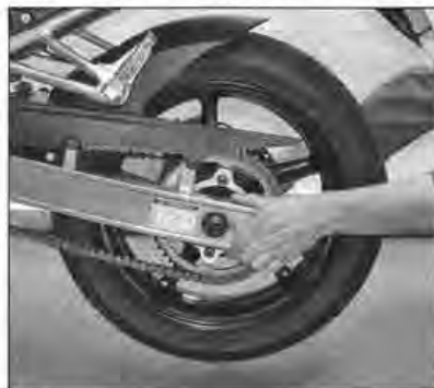
13.8 Checking for play in the swingarm bearings
