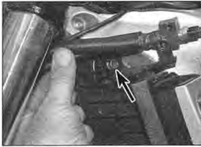
4.6c Displace the ABS pipe assembly to access the radiator top mounting bolt (arrowed)
