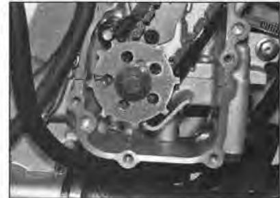
8.4b . . . to align the T mark with the rear facing crankcase mating surfaces
