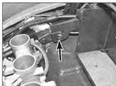
6.7a Press in the centre of the trim clip (arrowed) ...
