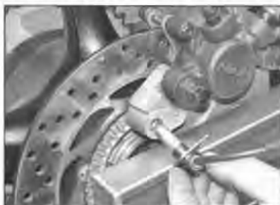
17.31b ... and draw the sensor out of the caliper bracket
