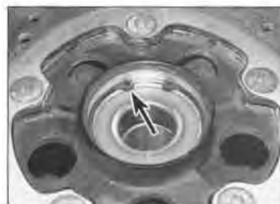
16.14a Remove the circlip from the right-hand side
