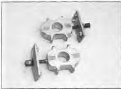
13.15 Check the chain adjusters for wear
