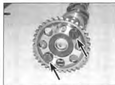
8.29 Camshaft sprocket bolts (arrowed)
