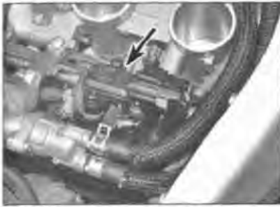
8.15 Location of the intake air pressure sensor (arrowed)
