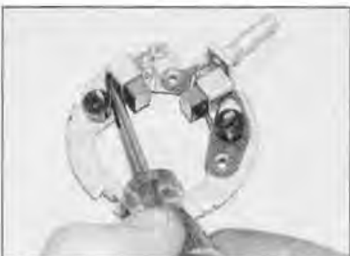
29.9 Move the brush springs aside and slide the brushes out
