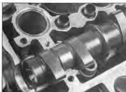
8.23 Lay a strip of Plastigauge across each bearing journal parallel with the centreline
