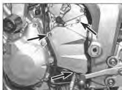
19.11a Remove the sprocket cover bolts (arrowed) ...
