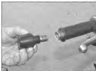
5.4a Unscrew the handlebar end-weight . . .
