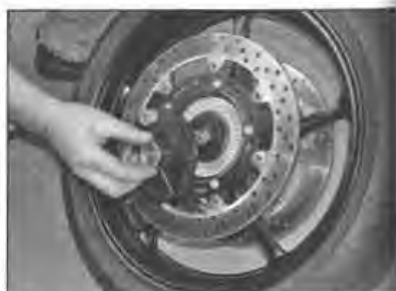
14.5b Remove the mounting plate for the ABS sensor
