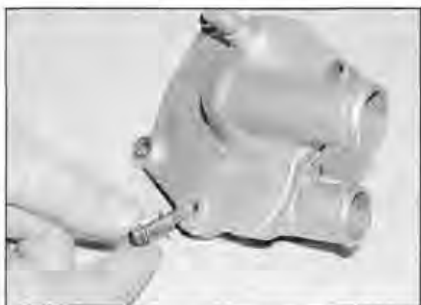
7.22 Fit a new sealing washer to the drain bolt
