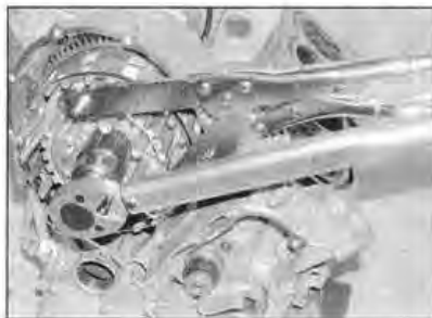
13.36c Tighten the clutch nut to the specified torque and secure it with the lockwasher tabs
