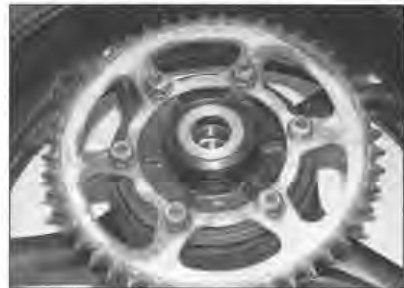
19.20 Rear sprocket is secured by six nuts
