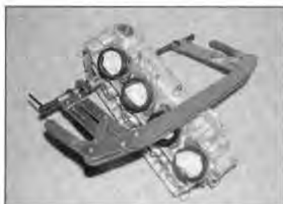
11.7a Compressing the valve springs using a valve spring compressor
