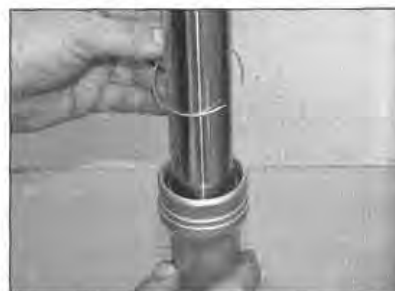
8.6b . . . carefully ease out the seal retaining clip
