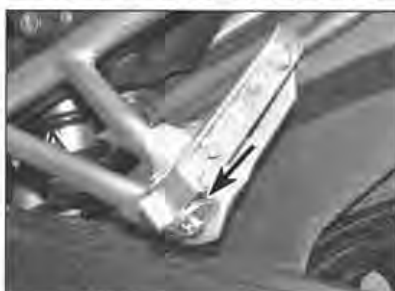
3.3 Note the location of the sprung ball (arrowed) on the passenger footrest
