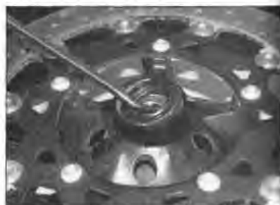
16.2 Lever out the bearing seals – front wheel
