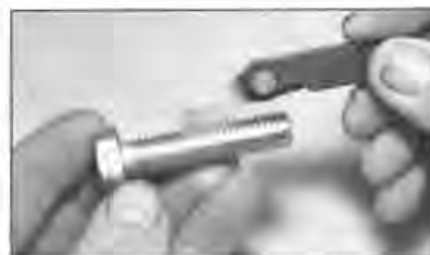
2.12 Using a thread gauge to measure pitch
