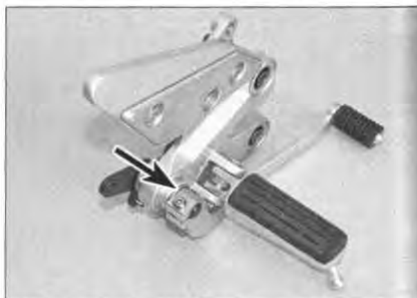
3.21 Note the location of the washer (arrowed) behind the brake pedal
