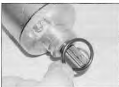
28.6 Ensure the new O-ring is correctly seated
