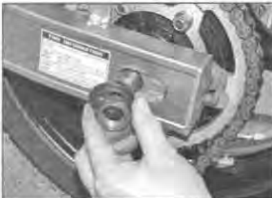
15.4a Remove the axle nut and washer
