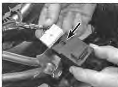
24.3b . . . then release the catch (arrowed) and disconnect the wiring connector
