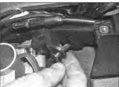
12.2c ... so that the clutch cable support bracket can be displaced
