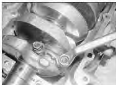
21.36d . . . and tighten them finally with a ring spanner as described
