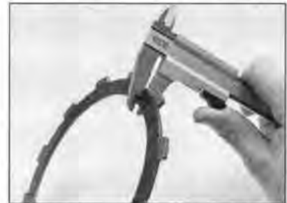
13.19 Measuring clutch friction plate thickness
