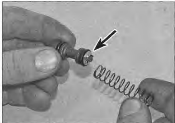
9.15 Push the end of the spring over the tabs (arrowed)
