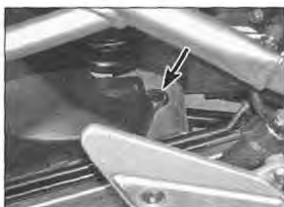
11.3b Release the centre of the trim clip (arrowed) ...
