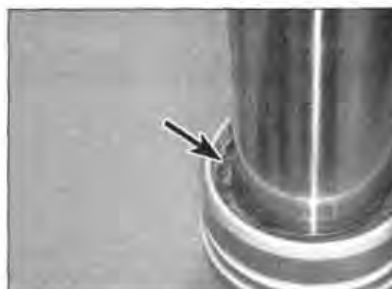
8.27 Ensure that the clip is located securely in its groove (arrowed)
