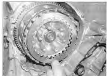
13.37a First install the thick plain plate ...
