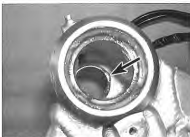
10.3a Locate the end of the drift in the cutout (arrowed) . . .
