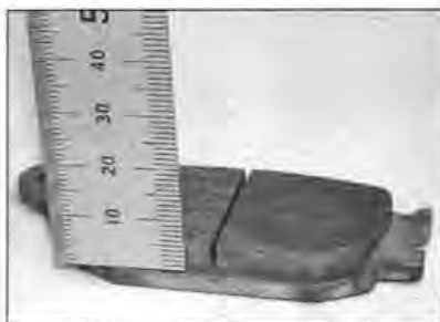
11.16 Measuring the thickness of the friction material
