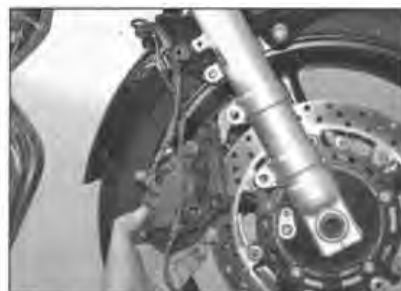
3.2c Slide the caliper assembly off the disc
