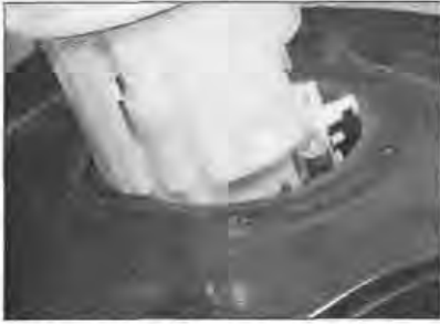
3.14 Position the pump as shown when fitting it into the tank
