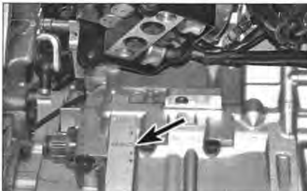
24.21a Main bearing size codes (arrowed)
