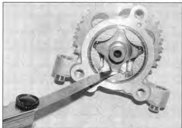
18.13 Measure the inner rotor tip to outer rotor clearance as shown
