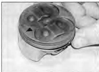
22.2 Note the arrow that points to the front of the engine
