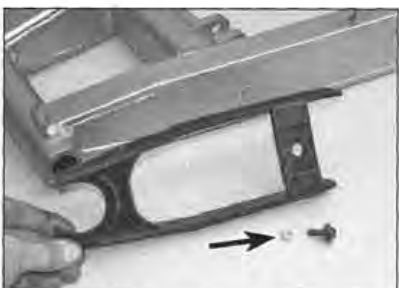
13.11 Note the small collar (arrowed) on the chain slider mounting screw
