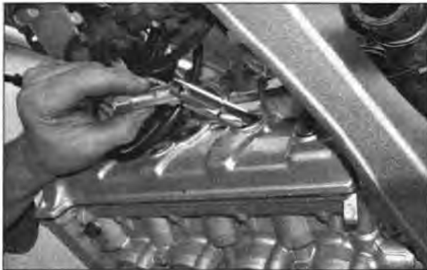
2.4a Insert the plug socket into the spark plug well – Yamaha tool shown ...
