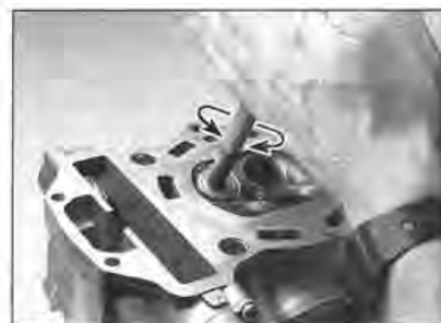
11.26a Rotate the valve grinding tool back and forth between the palms of your hands (arrowed)
