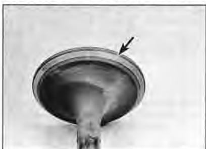
11.26b The valve face (arrowed) and seat should appear as a uniform, unbroken ring ...
