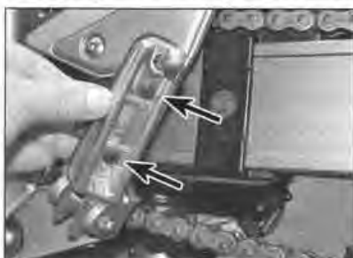
3.2 Footrest rubbers are secured by screws (arrowed) on the underside
