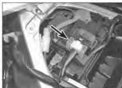
5.1a Location of the main fuse (arrowed) on the starter relay
