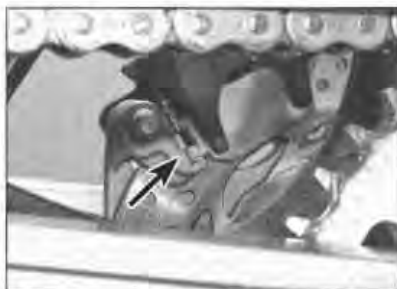
6.19b ... and inner pad locates against the pad plate (arrowed)
