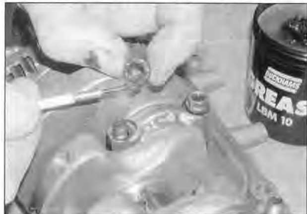
21.35 ... then install the cap nuts or bolts finger-tight
