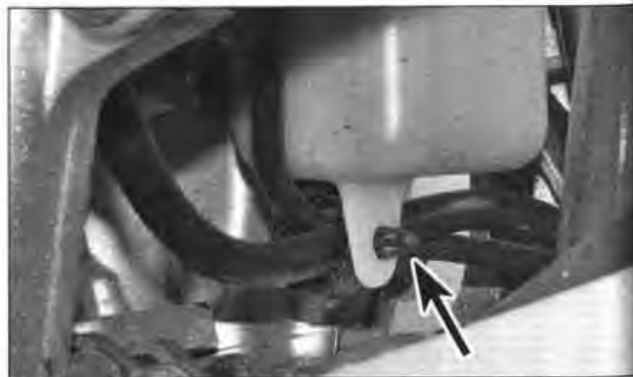
3.3a Release the clip (arrowed) securing the hoses ...
