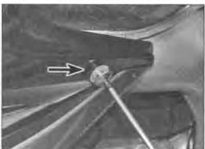
5.4b ... noting the location of the large washers (arrowed)
