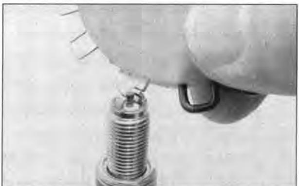
2.7c Adjust the electrode gap by bending the side electrodes only
