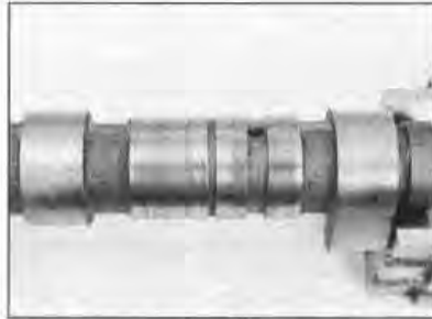
8.14 Check all related bearing surfaces as described
