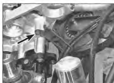
9.7b Bolt (arrowed) secures cable guide to top yoke
