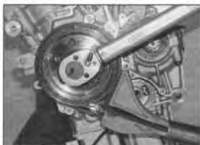
31.13 Tighten the rotor bolt to the specified torque
