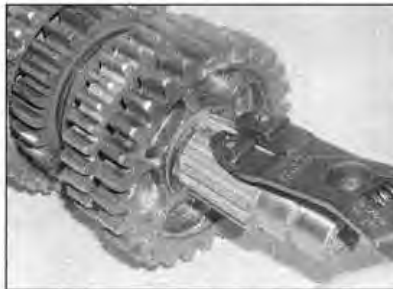
26.46d . . . and secure them with the circlip
