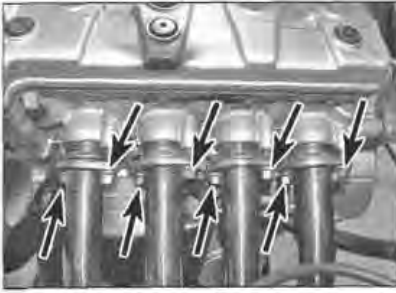
13.18a Unscrew the flange nuts (arrowed) ...
