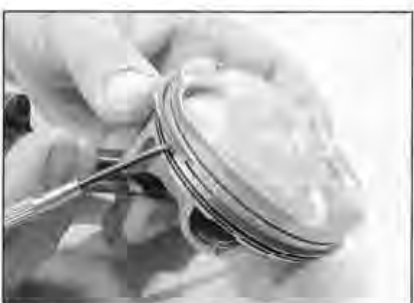
23.10a Carefully feed the second ring into its groove
