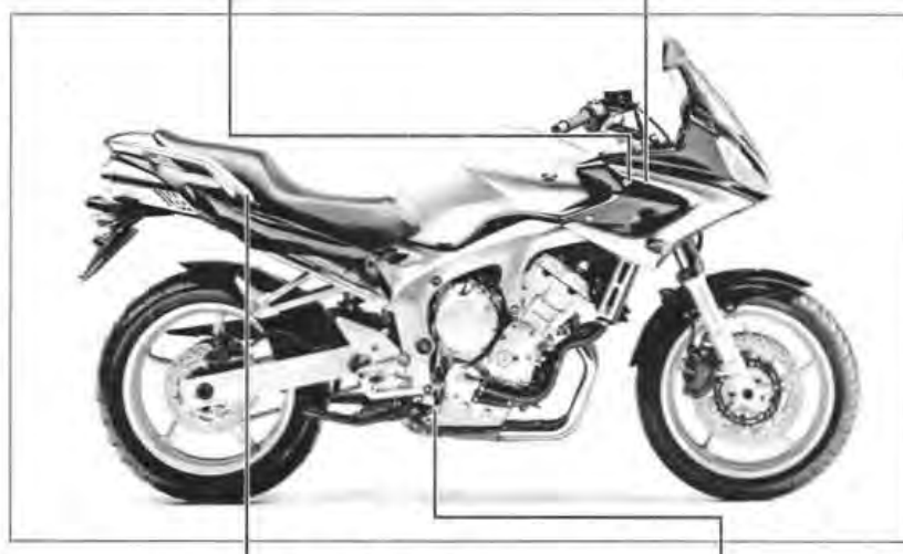
The frame number is stamped into the right-hand side of the steering head ...
