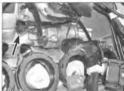
8.49 Undo the screw (arrowed) to remove the speed sensor
