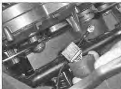
5.10b . . . and disconnect the multi-pin wiring connector
