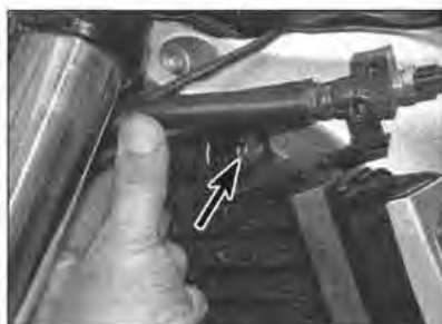
2.8c Displace the ABS pipe assembly to access the radiator top mounting bolt (arrowed)
