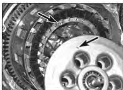
13.10a Note the alignment marks (arrowed)
