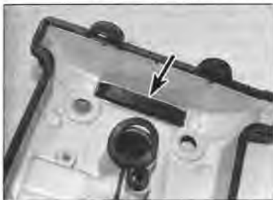
9.1 The top guide (arrowed) is fixed in the valve cover
