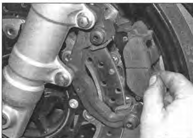
11.11b . . . but a better assessment can be made with the caliper displaced
