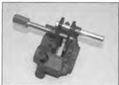
2.9b Set-up using a commercially available piston retracting tool
