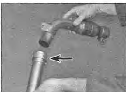
13.8a Note the location of the sealing ring in the silencer front pipe (arrowed) ...
