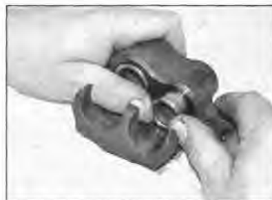
3.16b Push the pistons in squarely using hand pressure
