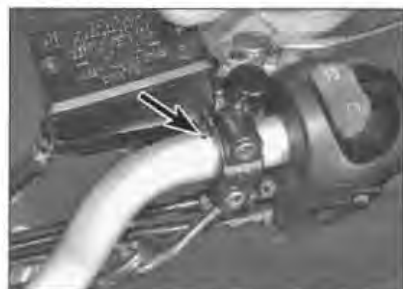
5.14b Align the clamp mating surfaces with the punch mark (arrowed)
