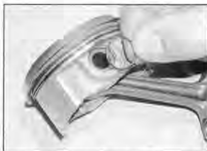
22.15 Fit the circlip with the open end away from the removal notch
