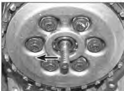
13.43 Pull-rod teeth should face rearwards
