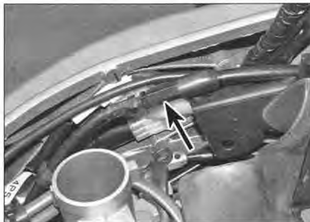
7.8 Location of lower clutch cable adjuster (arrowed)
