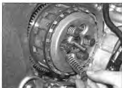
13.9 Remove the clutch bolts and springs
