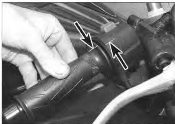
6.4 Throttle cable freeplay is measured in terms of twistgrip rotation
