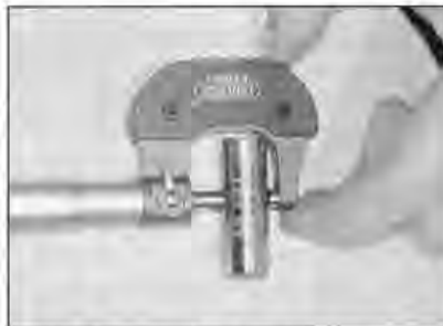
21.10b Measure the diameter at the centre of the pin
