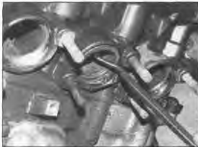
13.22 Remove and discard the old exhaust port gaskets
