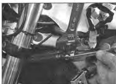
2.8b Hold the union to prevent it twisting while undoing the mounting bolt
