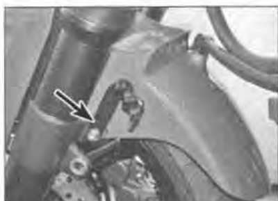
7.5 Install the brake hose bracket on the left-hand side (arrowed)
