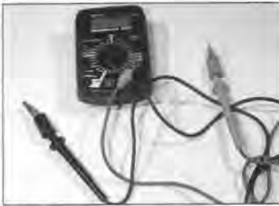
2.4a A digital multimeter can be used for all electrical tests
