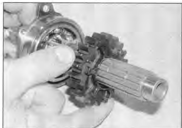
26.20b ... the 5th gear pinion ...
