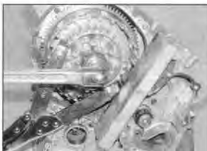
13.12b Remove the clutch nut as described
