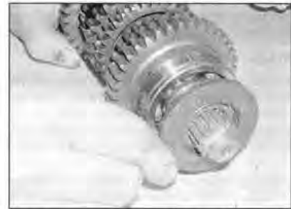
25.3b . . . and discard the shaft oil seal
