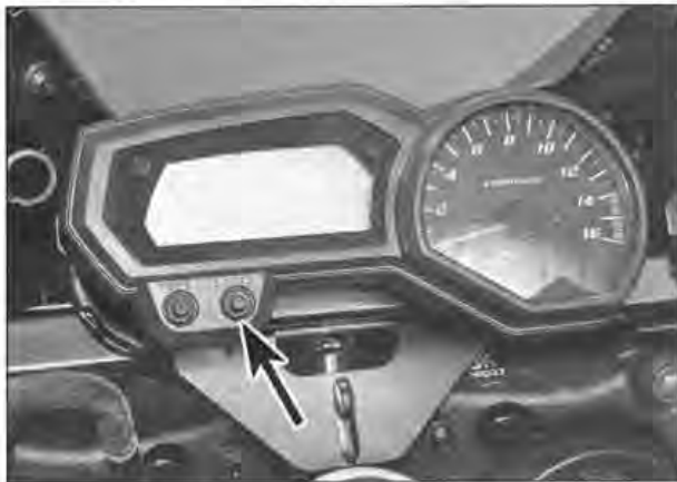
15.10a SELECT button (arrowed) – S2 models
