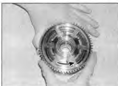
14.8 Check that the driven gear turns freely anti-clockwise
