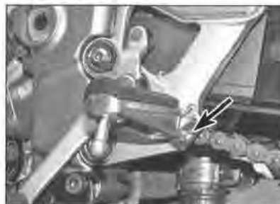
3.1a Remove the split pin (arrowed) . . .
