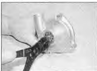
7.16 To remove the bearing, first remove the circlip
