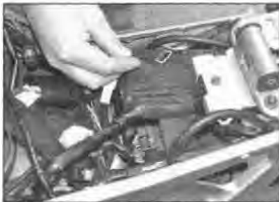
17.107a Release the holding strap ...
