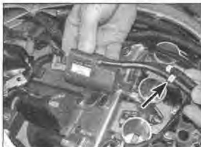
17.11 Lift out the upper ignition coil. Note the numbered HT leads (arrowed)
