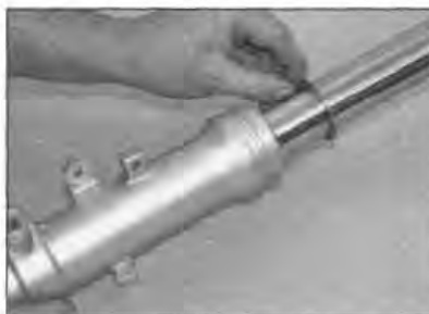
8.24b . . . then slide on the washer
