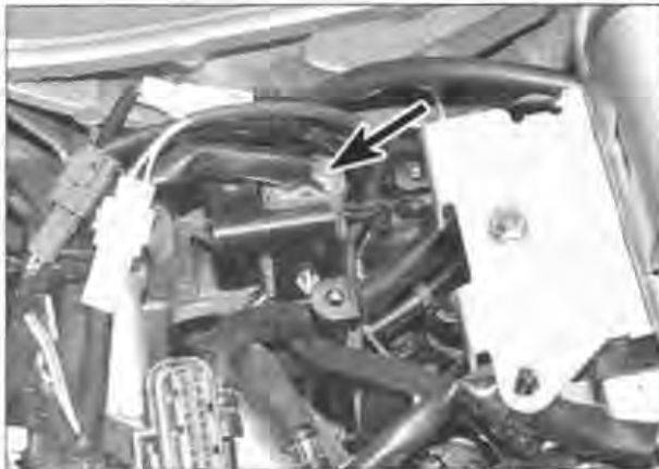
17.61 Location of the modulator motor wiring connector (arrowed)
