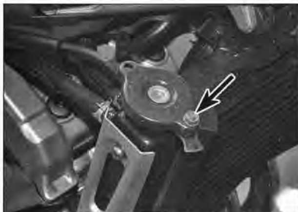
9.13b Don't forget to tighten the lock bolt (arrowed) securely
