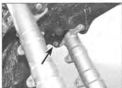
7.8b Rear screws (arrowed) are installed from the inside
