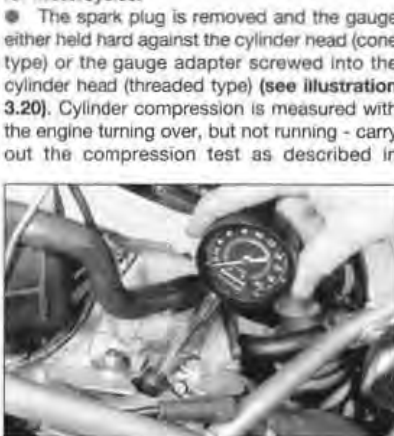
3.20 Using a rubber-cone type cylinder compression gauge
