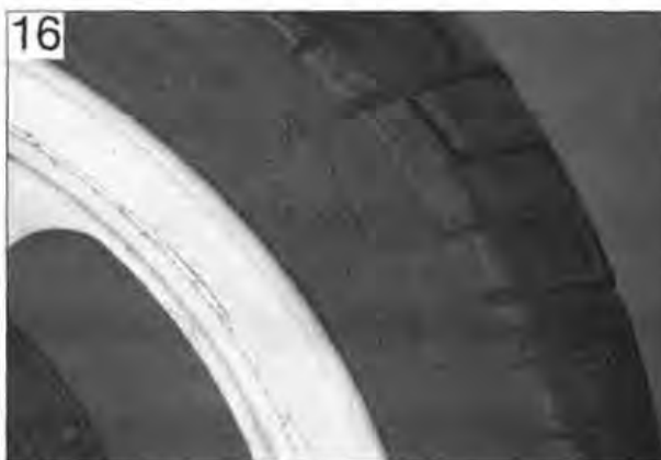
Tyre direction of rotation arrow can be found on tyre sidewall
