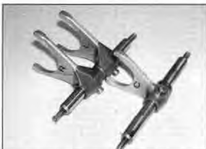
27.4 Note the letter on each fork denoting its position
