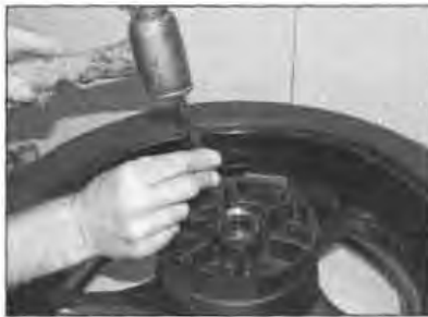
16.14c Using a metal rod to drive the bearing out
