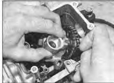
18.6 . . . then disengage the chain and remove the pump
