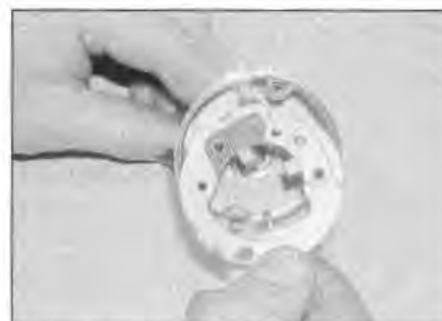
29.8a Remove the brushplate from the cover . . .
