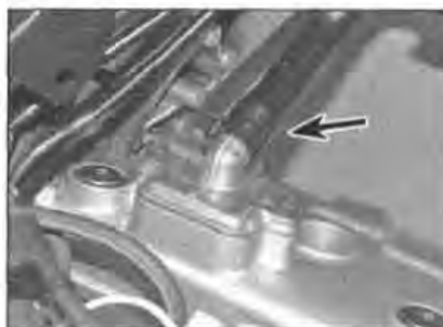
14.6 Release the clip before pulling the hose off the union (arrowed)
