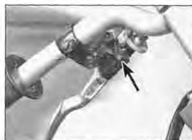
23.4 Clutch switch is secured by single screw (arrowed)
