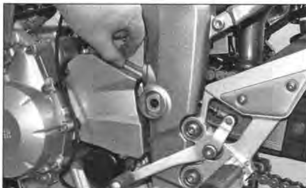
15.1c . . . then unscrew the rod and withdraw it from the frame
