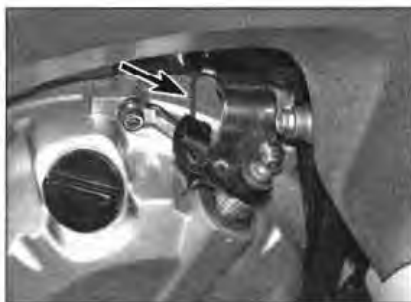
12.3b ... to obtain freeplay in the inner cable (arrowed)
