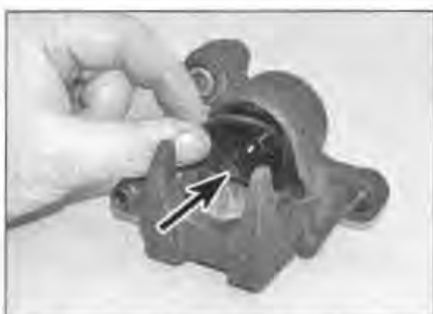
7.12 Fit the new piston seal and dust seal into the appropriate grooves (arrowed)
