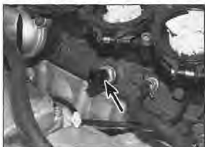
5.13 Unscrew the temperature sensor (arrowed) from the rear of the cylinder head
