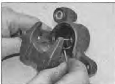
7.8 Remove the old seals carefully to avoid damage to the bore and seal groove
