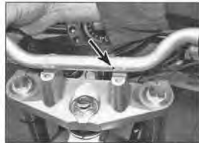
5.12 Check the alignment of the register mark (arrowed)
