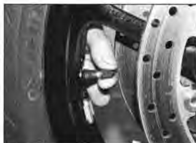
12.2a Make sure there is a cap on each valve
