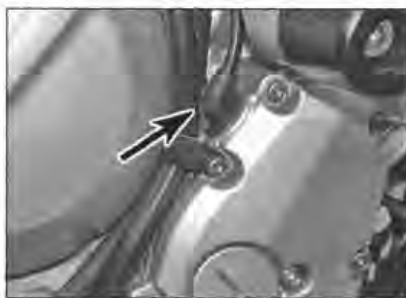
8.5a Trace the crankshaft position sensor wiring (arrowed) . . .
