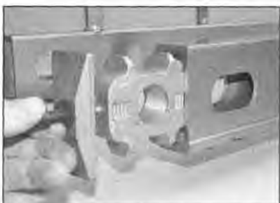
13.9 Remove the chain adjusters for safekeeping
