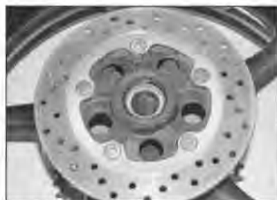
8.4 The brake disc is secured by five bolts
