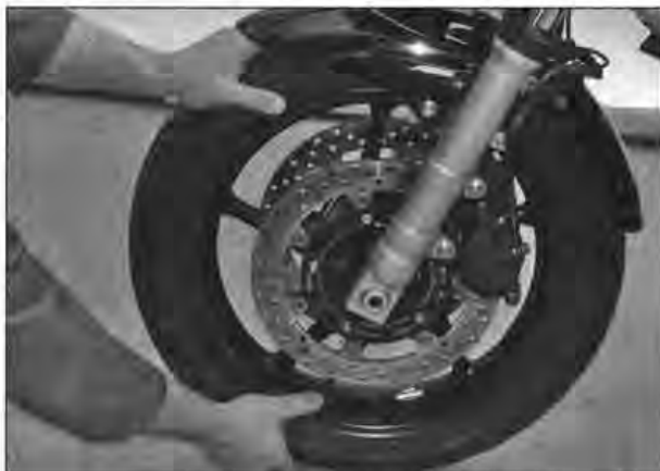
12.5 Checking for play in the wheel bearings
