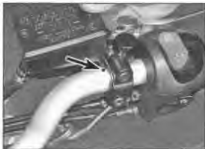
5.4a Note the alignment of the clamp with the register mark (arrowed)
