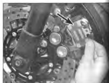
2.21 Withdraw the pads, noting the location of the anti-chatter shims (arrowed)
