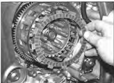
13.37d ... followed by a brown-coded friction plate
