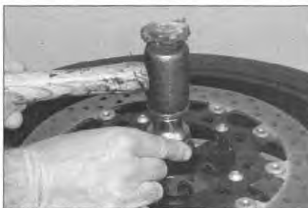
16.7 Using a socket to drive the bearing in
