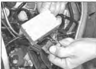
17.109 Press the catch down to release the connector
