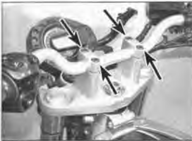
5.11a Loosen the clamp bolts (arrowed)
