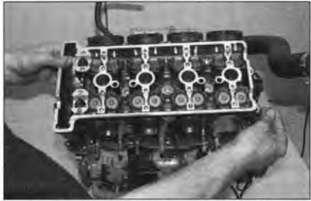
10.4 Lift the head up off the block and remove it
