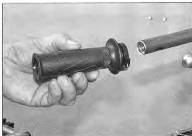
6.3c . . . then slide the twistgrip off
