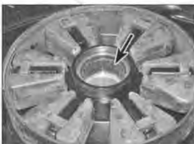
16.13b ... to inspect the bearing needle rollers (arrowed)
