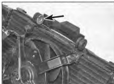
2.11a Check the condition of the mounting bushes. Note the spacer (arrowed)
