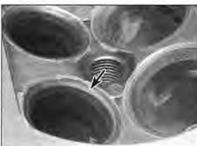
11.26c ... and the seat (arrowed) should be the specified width all the way round
