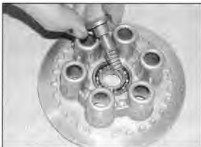
13.39 Fit the pull-rod into the back of the pressure plate
