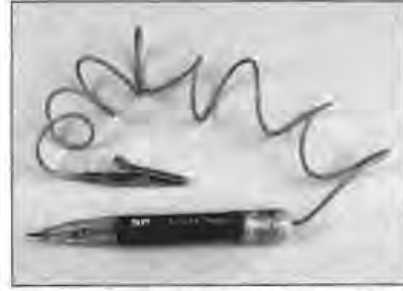
2.4c A simple test light can be used for voltage checks
