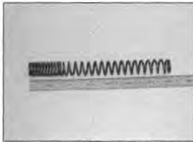
8.14 Measure the free length of the fork spring
