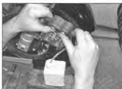
2.11b Open the valve and press the pistons into the caliper
