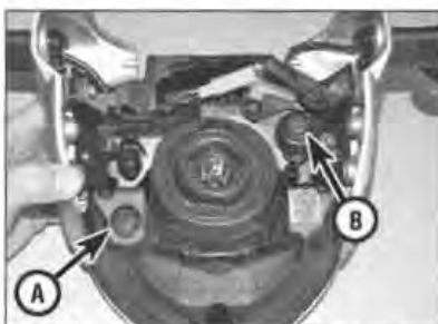
8.12 Vertical adjuster screw (A) and horizontal adjuster screw (B)
