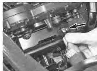
5.10c Release the earth wire from the bracket
