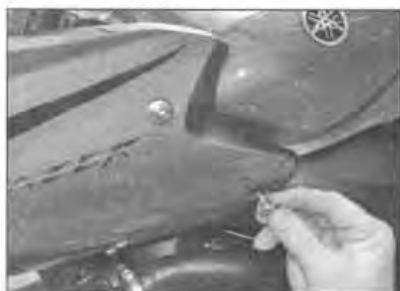
5.1a Undo the screws, noting the location of the large washers
