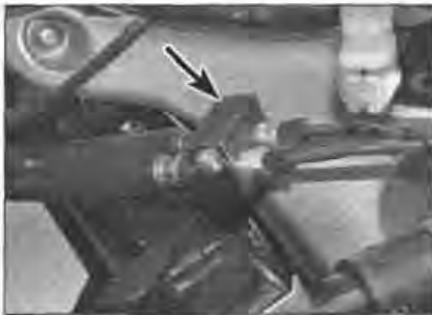
10.4a Brake hose/pipe union located on the left-hand side above the radiator
