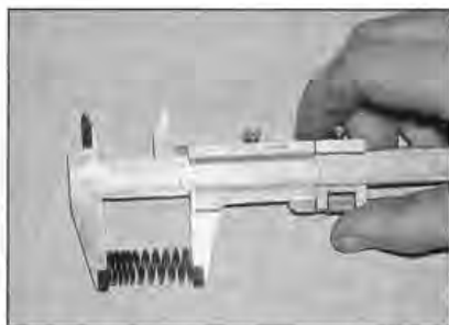
11.21 Measuring spring free length with a Vernier caliper
