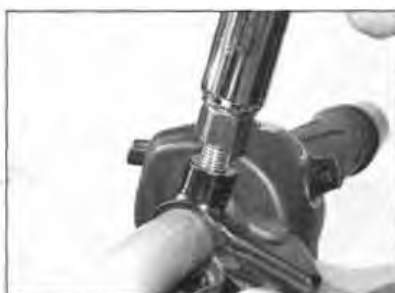
4.2 Take care when installing the mirror stem threads
