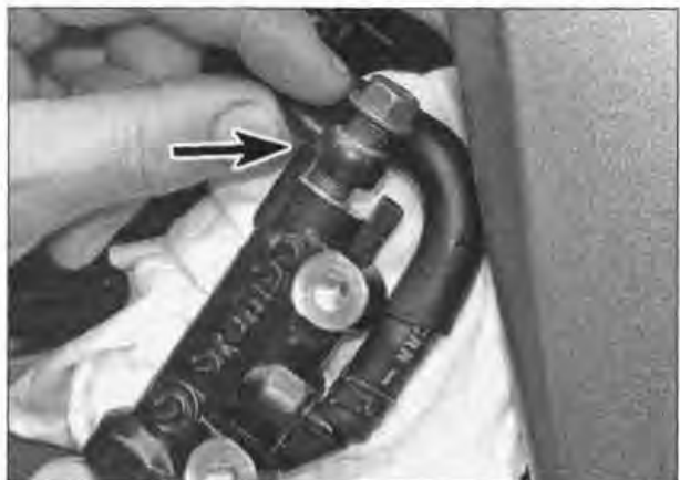
9.22a Banjo fitting locates in front of the tab (arrowed)
