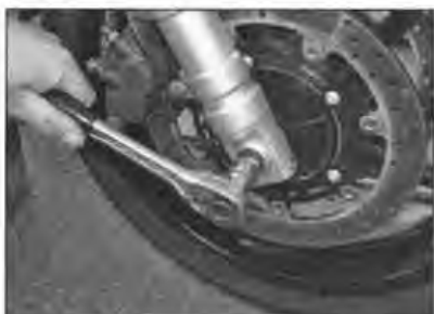
14.3c ... to slacken the axle
