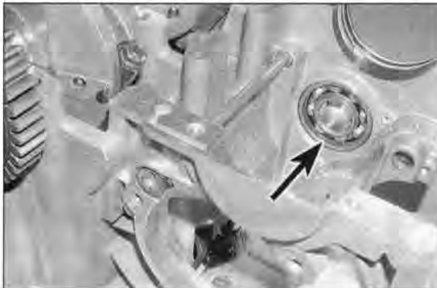
25.7a Locate the end of the input shaft in the bearing (arrowed)
