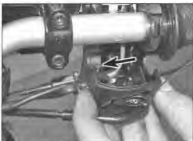
5.14c Peg (arrowed) locates in hole in the underside of the handlebar
