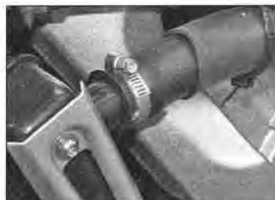
9.3 Ensure the hose clips are tightened securely
