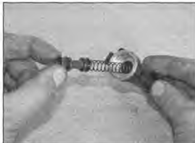
9.10c ... the piston and the spring
