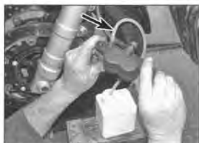
2.11a Attach a length of hose to the bleed valve (arrowed)
