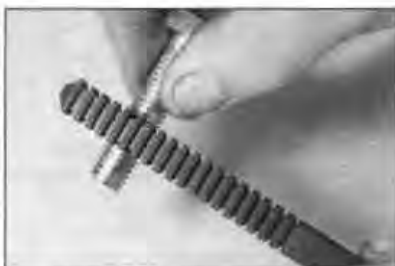
2.24 Using a thread restorer file
