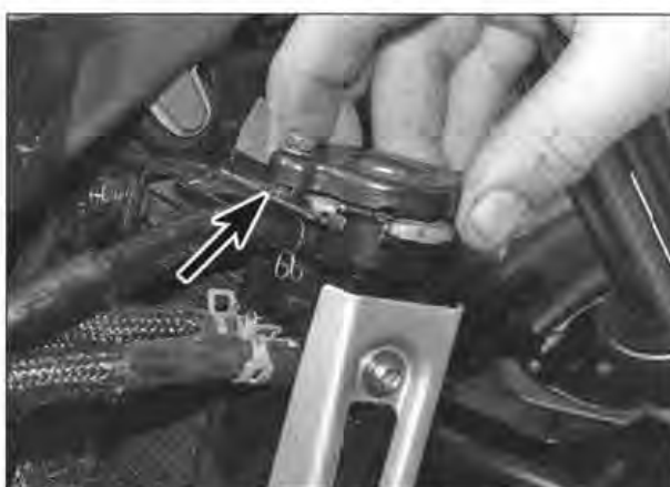
9.13a Check the position of the locking tab (arrowed) before fitting the cap
