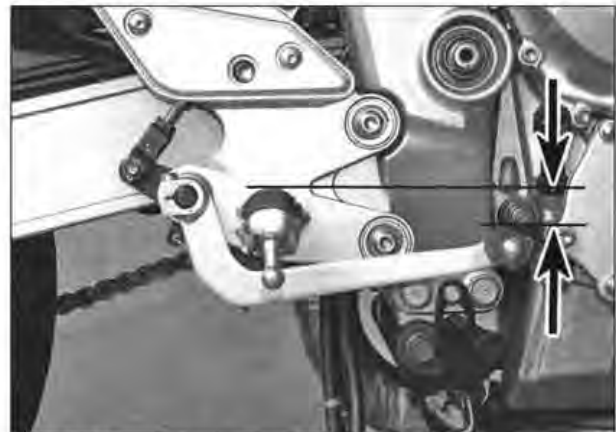
11.10a Measure the brake pedal height between the two points (arrowed)
