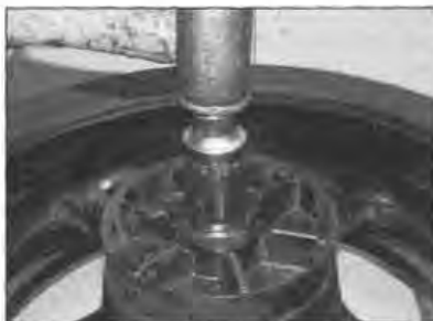
16.17 Using a suitable socket to drive the caged ball bearing in
