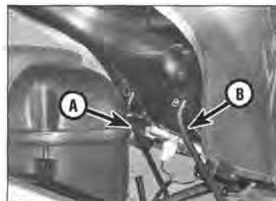
2.5 Detach the breather hose (A) and drain hose (B)
