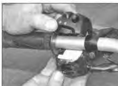
20.5a Separate the halves of the switch unit
