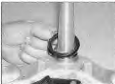
9.15b . . . and the dust seal from the steering stem
