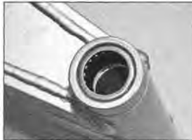
14.3 A needle roller bearing is located at each end of the pivot tube
