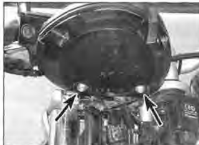
15.3c Undo the instrument cluster bracket screws (arrowed) ...
