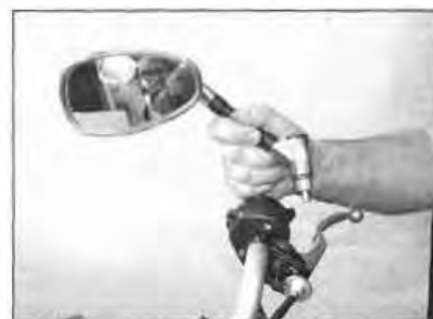
4.1b ... then unscrew the mirror
