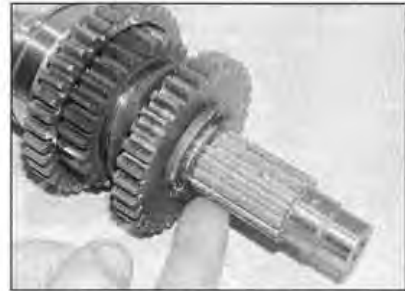
26.45 . . . then slide on the tabbed lockwasher
