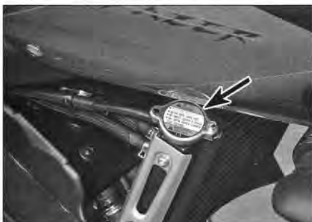
9.18b Location of the radiator pressure cap – S2 models
