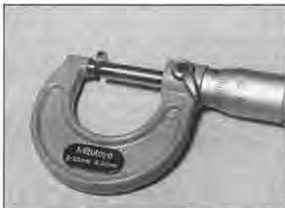
19.16 Measuring the shim with a micrometer
