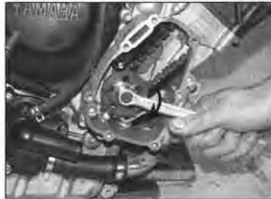
8.4a Turn the engine clockwise using the rotor bolt . . .
