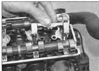
8.10 Unscrew the bolts as described and remove the holders
