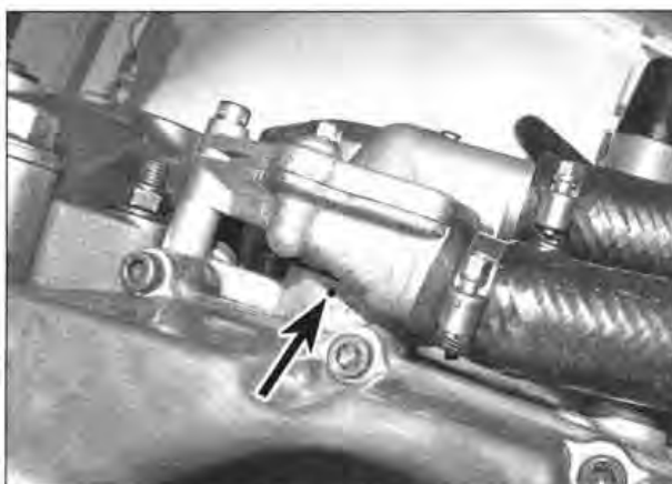
9.6 Check for signs of leakage from the pump drain hole (arrowed)
