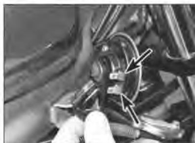
25.3 Pull the connectors off the horn terminals (arrowed)
