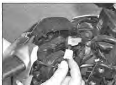
8.3 Disconnect the turn signals wiring connector
