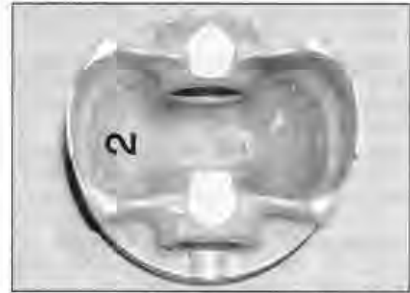
22.7b . . . and that the piston is still clearly marked
