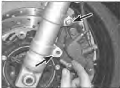
3.1b Undo the caliper bracket bolts (arrowed) ...
