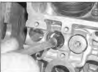
11.29b Press the new stem seal into place with a suitable deep socket
