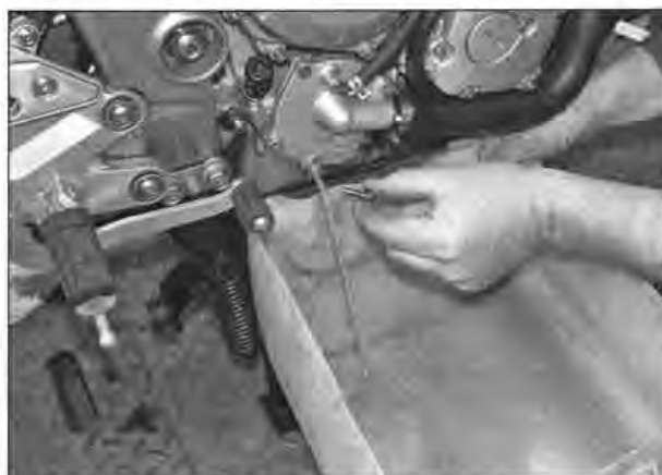
9.19 Draining the coolant from the water pump drain hole
