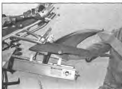
11.3e ... and lift the hugger/chainguard off
