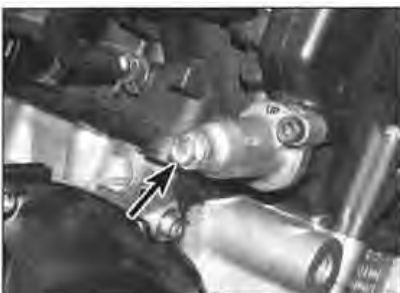
7.3 Unscrew the cap bolt (arrowed) and remove the washer
