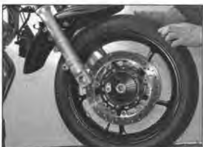
14.4b Remove the wheel
