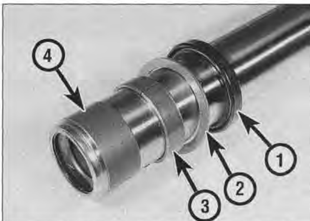
8.8b . . . the slide-hammer effect of the bottom bush (4) will displace the top bush (3), washer (2) and oil seal (1)
