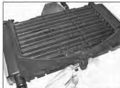
2.11b Ensure the spacers are fitted before assembly
