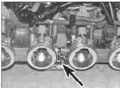
9.19b Ensure that the throttle linkage is clean (arrowed)
