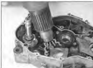
2.15 Using heat to free a seized fastener
