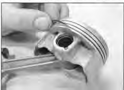
23.8a Fit the oil ring expander in its groove ...
