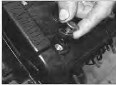
6.8 Use new sealing washers with the bolts if necessary
