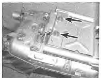
13.6 Undo the silencer mounting bolt (arrowed)
