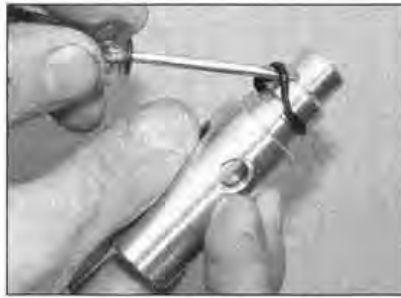
17.9 Fit an new O-ring and lubricate it
