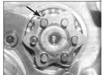
27.3 Note the position of the neutral detent (arrowed) on the end of the selector drum
