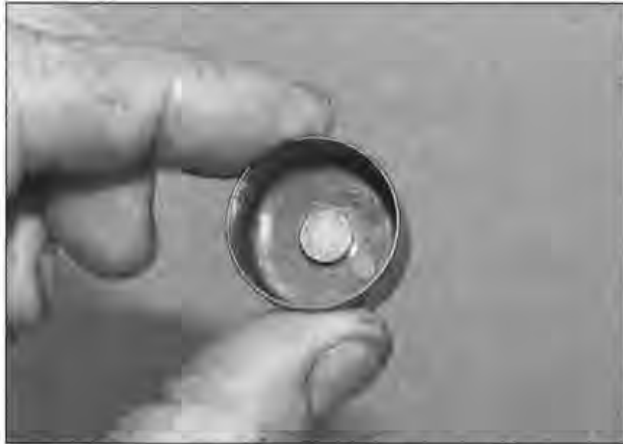
19.15b ... and retrieve the shim from inside ...
