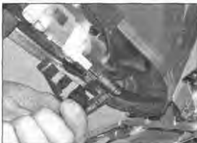
2.7a Remove the security clip . . .
