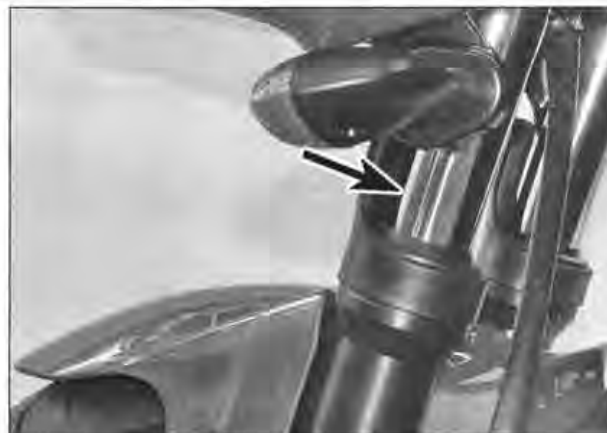
13.3 Inspect the fork inner tubes for surface damage and oil leakage
