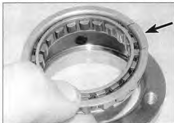
14.9b Depress the spring lock (arrowed) to release the clutch assembly from its housing
