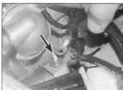
28.3 Detach the lead from the starter motor terminal (arrowed)
