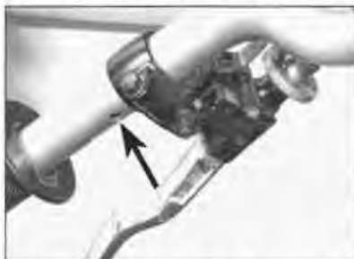
20.5c . . . locates in the hole (arrowed) in the handlebar
