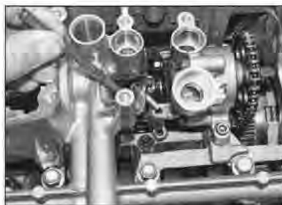
18.21a Fit the oil return pipe ...
