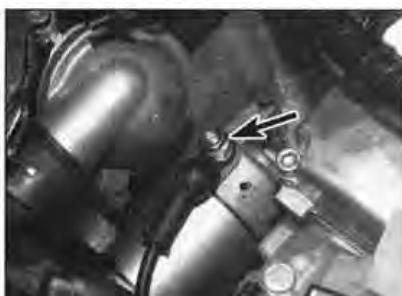
4.14 Detach the lead from the starter motor terminal (arrowed)
