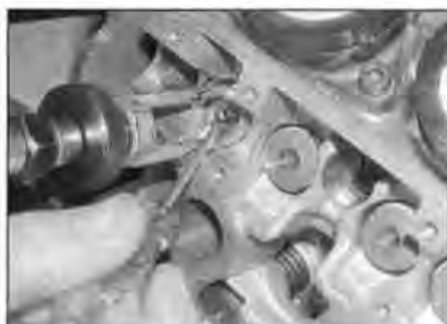
11.8a Remove the collets taking care not to drop them into the engine
