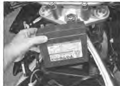
3.6 Lift the battery out of its housing
