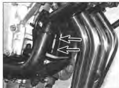
2 . . . or below the radiator. The coolant FULL and LOW level lines (arrowed) are marked on the reservoir.
