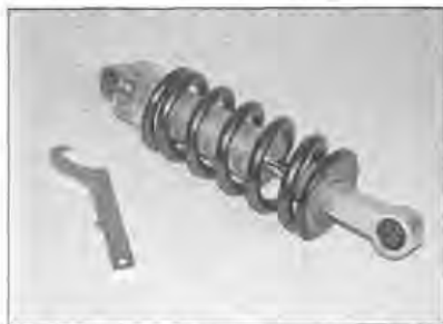
12.2 A spanner is provided in the toolkit for pre-load adjustment
