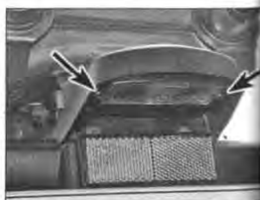
9.6 Undo the screws securing the licence plate light unit
