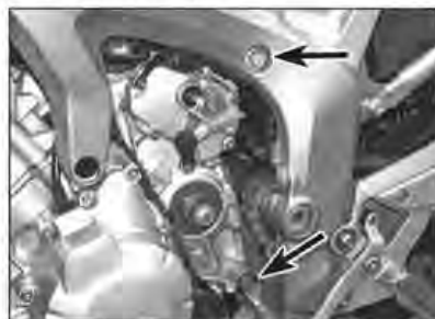
4.24c ... then withdraw the bolts (arrowed)
