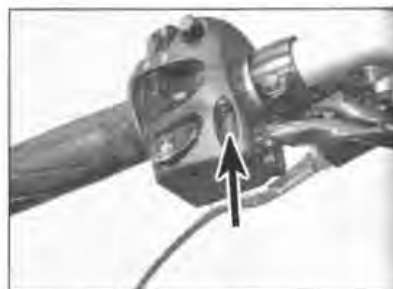
20.4b . . . and rear (arrowed) left-hand switch unit screws
