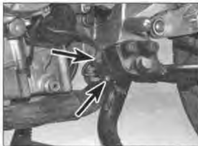
4.3a Undo the screws (arrowed) to displace the stand switch ...
