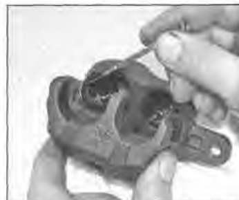
3.10 Remove the seals carefully to avoid damage to the bore and seal groove
