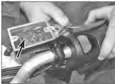
11.5 Check for air bubbles (arrowed) in the brake fluid
