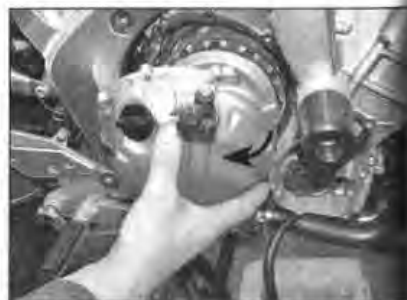
13.44 Release arm should turn rearwards as the cover is installed
