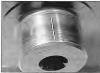
24.12 Place a strip of Plastigauge on each bearing journal
