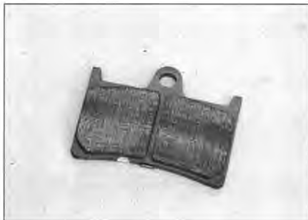
11.15 Note the two separate sections of friction material bonded to the backplate
