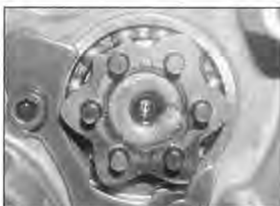
15.9 Check the selector pins for wear
