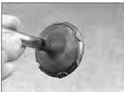
11.25 Apply small dabs of grinding compound to the valve face only
