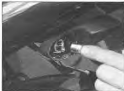
12.4 Pins on the bulb must align with slots in the bulbholder
