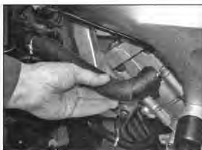
4.13b ... and pull the hose off
