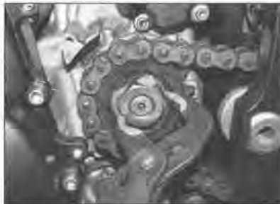
19.16 Lock the nut by bending the lockwasher against it
