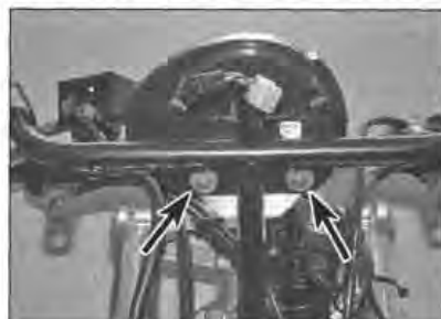
15.8b Instrument cluster on all other S models is secured by two screws (arrowed)
