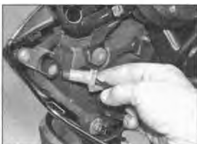
7.19a Draw the bulbholder out ...
