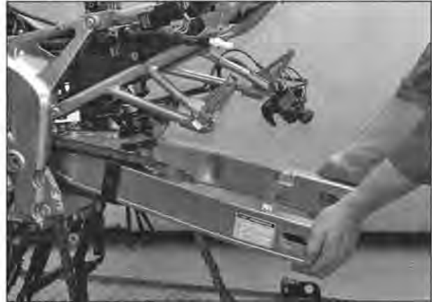
13.11 Swingarm should move freely up and down
