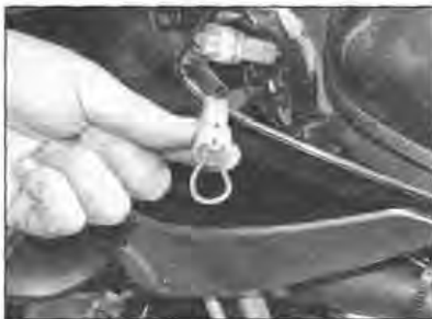
11.11c ... and join the light blue and black wire terminals
