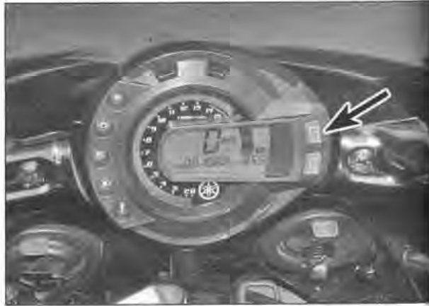
15.10b SELECT button (arrowed) – all other S models
