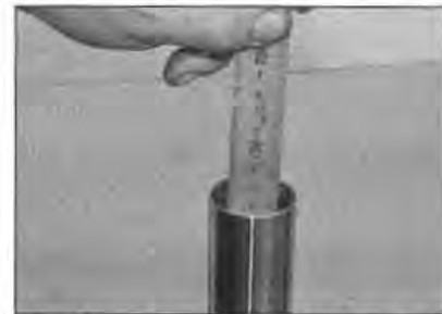
7.7 Measure the oil level with the leg fully compressed
