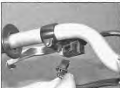
5.7 Disconnect the clutch switch wiring connector
