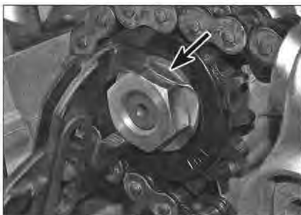
1.21 Ensure that the lockwasher is folded over against a flat (arrowed) on the sprocket nut
