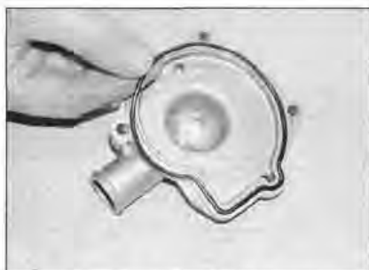
7.8 Note how the seal fits in the cover
