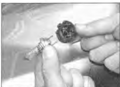
7.14c Pull the headlight bulb out of its holder
