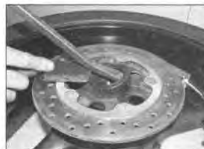
16.12 Lever out the bearing seal – rear wheel
