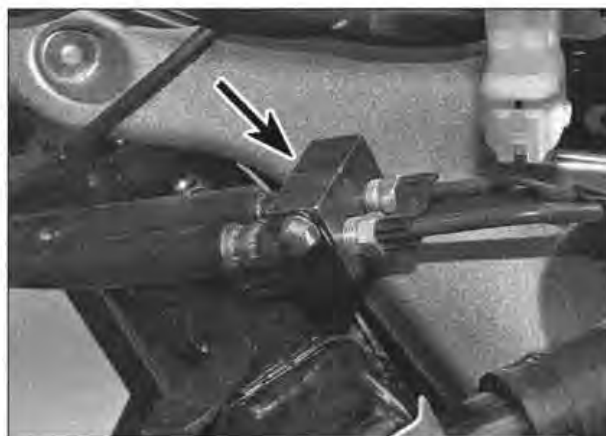
2.8a ABS pipe assembly is secured to radiator bracket through this union (arrowed)
