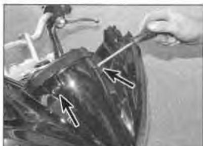
5.18 Remove the two screws (arrowed)
