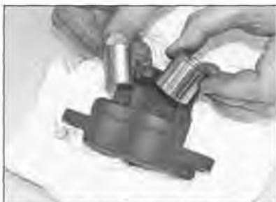
3.8 The pistons are different sizes – mark their locations in the caliper
