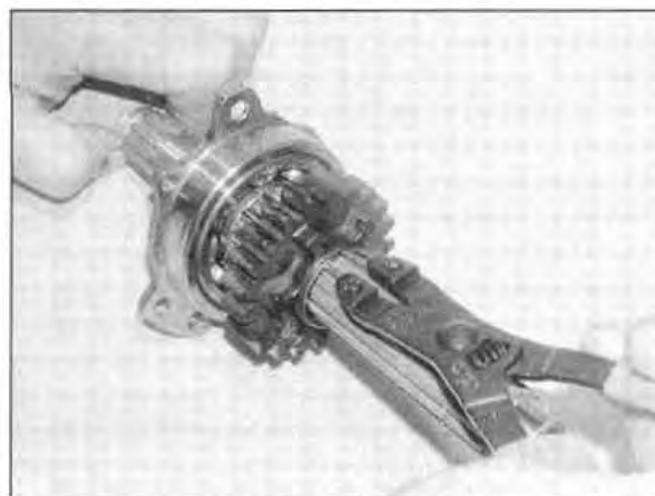
26.21b ... and secure them with the circlip
