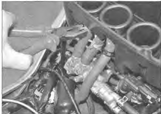
5.2b Release the hose clips with pliers
