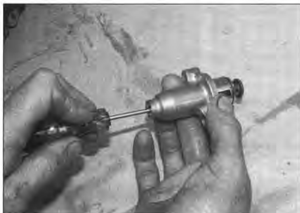
7.7 Check the action of the plunger as described
