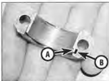
21.15 Ensure tab (A) locates in notch (B)
