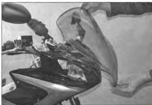
3.5b ... then lift the windshield off
