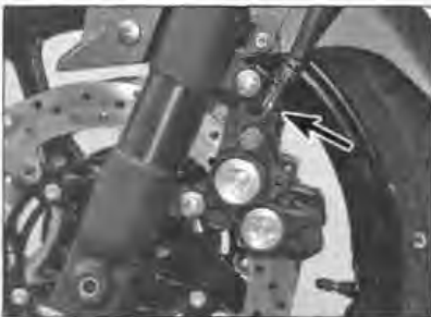
3.29 Note the alignment of the banjo fittings (arrowed)
