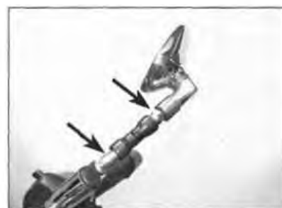
4.3 Final adjustments can be made at the joints (arrowed)
