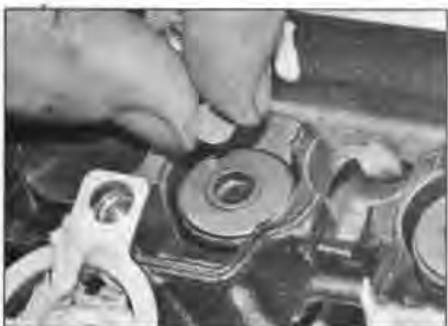
8.31 Fit each shim into its recess
