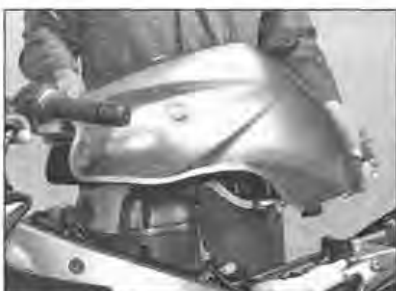
2.8 Remove the rear bolt and lift off the tank
