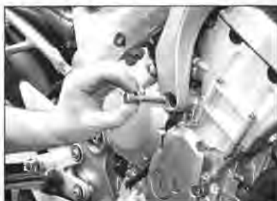
4.22 Unscrew the right-hand front mounting bolt
