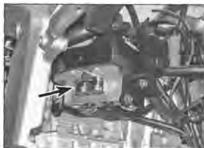
17.43a Location of the ABS modulator solenoids (arrowed)
