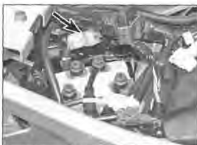
17.43b Location of the solenoid wiring connector (arrowed)
