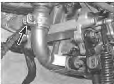
13.2 Slacken the clamp bolt (arrowed) at the rear of the header pipe assembly
