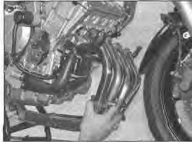
13.21a Detach the header pipes from the cylinder head ...
