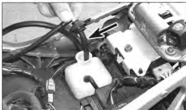
3.2 Remove the cap and draw out the end of the overflow hose (arrowed)
