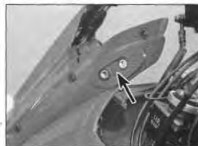
4.6 Note the location of the pad and collars (arrowed) – S2 models
