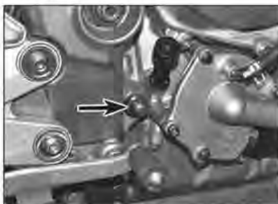
4.24b ... and lower (arrowed) rear mounting bolts ...
