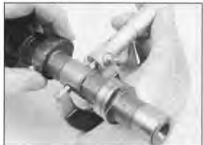
8.19 Measure the journals with a micrometer
