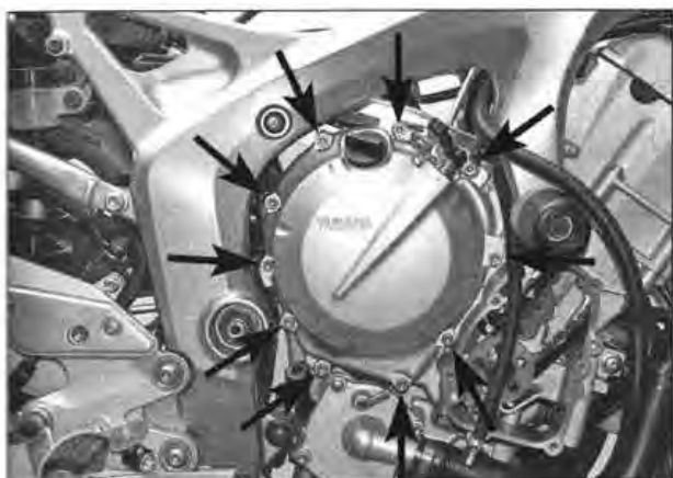
13.5a Unscrew the clutch cover bolts (arrowed) ...
