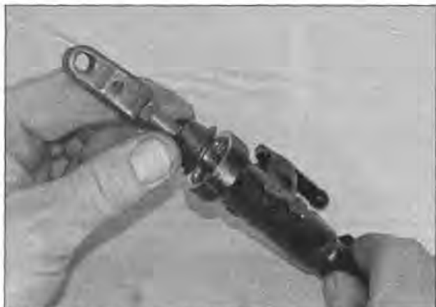
9.17 Push the boot down into the end of the master cylinder
