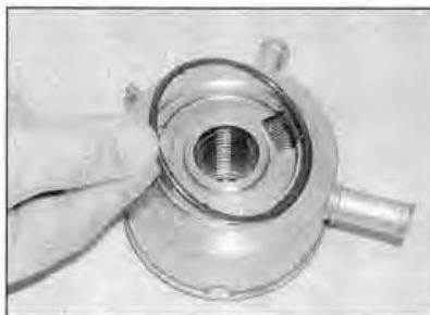
16.7 Use a new O-ring on the oil cooler body
