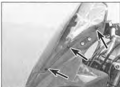
3.1 The windshield is secured by three screws on both sides – S2 models
