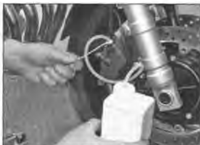
11.2a Set-up for bleeding the front . . .
