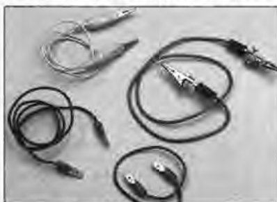
2.23 A selection of jumper wires for making earth (ground) checks
