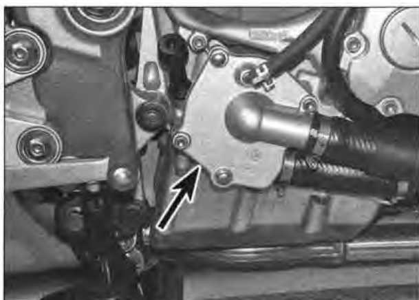
9.5 Location of the water pump (arrowed)
