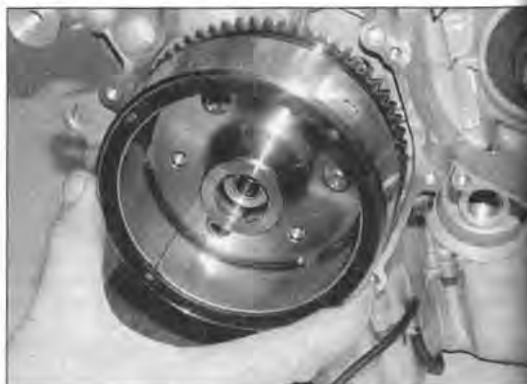
31.12 Slide the rotor onto the crankshaft
