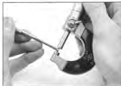
3.10 ... then measure the gauge with a micrometer
