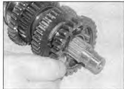
26.46b . . . then slide on the 3rd gear pinion . . .
