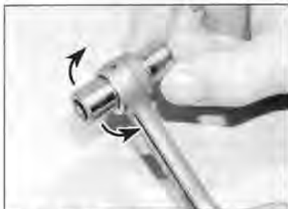
21.10a Rock the piston pin back and forth in the small-end to check for looseness (arrowed)
