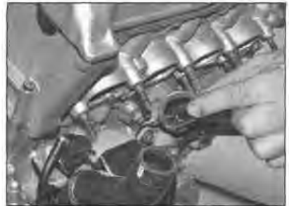
13.25 Secure the new exhaust port gaskets with a smear of grease
