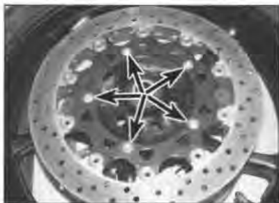
4.5 Undo the bolts (arrowed) and remove the disc
