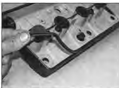
6.7a Fit the gasket into the groove in the rim of the cover ...
