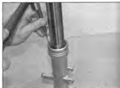
8.25 Installing the top bush with a pin punch and hammer
