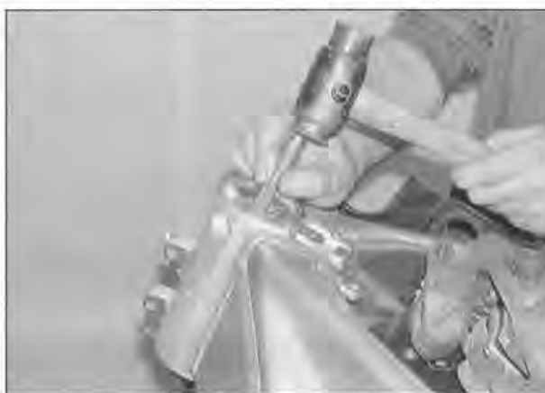
10.3b . . . and drive the race out
