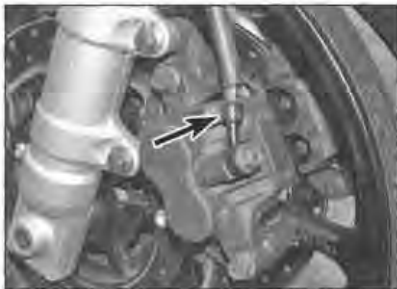
3.3a Note the alignment of the brake hose banjo fitting (arrowed)
