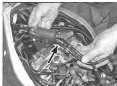
17.2a Ensure that the HT leads (arrowed) are secure
