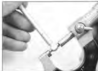
3.8 ... then measure the gauge with a micrometer
