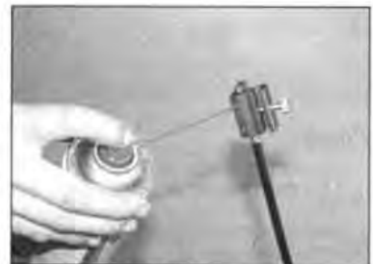
8.5c Apply the lubricant using the nozzle provided inserted into the hole in the adapter
