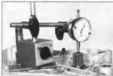
3.19 Using a dial gauge to measure shaft endfloat
