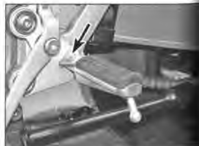
3.1b . . . then withdraw clevis pin (arrowed)
