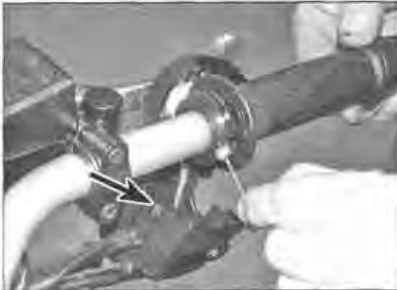
12.10a Detach the inner cable ends from the pulley. Note the locating pin (arrowed)
