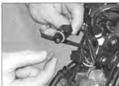
7.8 Pull the sidelight bulb out of its holder
