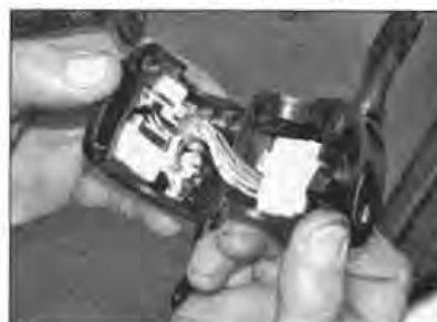
19.6 Keep the switch terminals clean and free from corrosion
