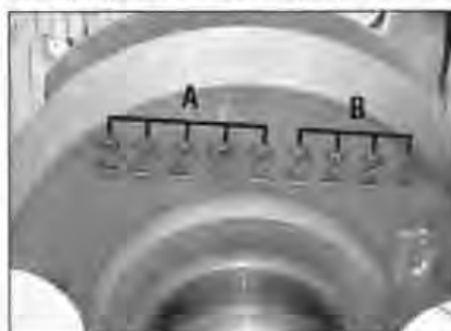
21.25a Main bearing journal numbers (A) and big-end bearing journal numbers (B)
