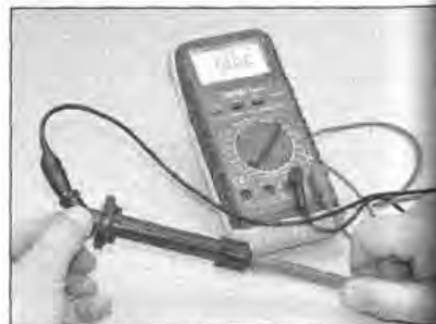
17.3b ... and check the plug cap resistance
