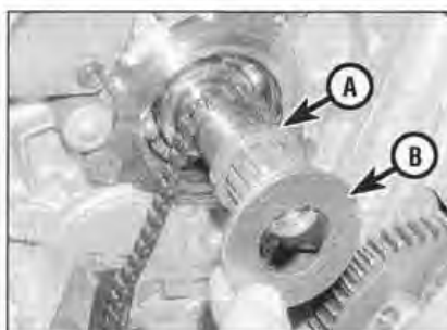
13.33a Install the spacer (A) and thrust washer (B)
