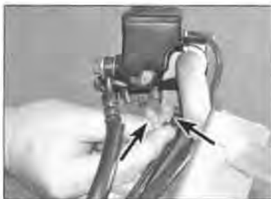
5.2 Disconnect the brake light switch wiring connectors (arrowed)
