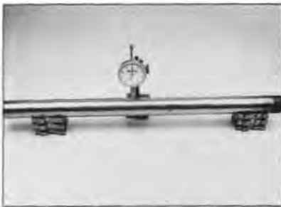
8.13 Check the inner tube for run-out using V-blocks and a dial gauge
