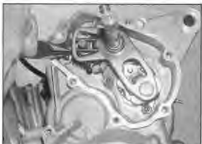
15.18 Hook the stopper arm spring over its anchor pin
