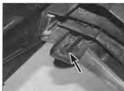
13.11 Unclip the mounting plate (arrowed) to release the turn signal assembly
