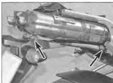
7.14a Undo the bolts (arrowed) on both sides . . .
