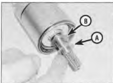
29.4b . . . and the insulating washer (A) and shim(s) (B)
