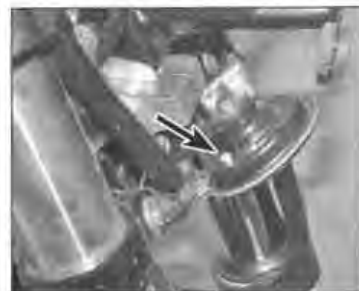
25.4 Screw (arrowed) for adjusting tone of the horn
