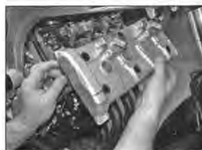
6.3c ... then lift the cover off
