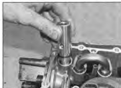
17.5 Pull the pressure relief valve out of its socket
