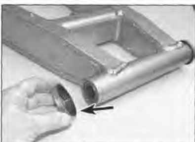
13.10 Check the seal (arrowed) inside both bearing end covers
