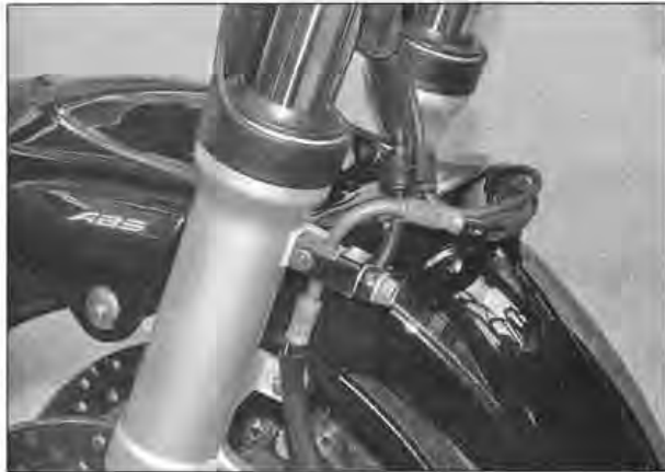
11.5 Inspect the brake connections and hoses for cracks and leaking fluid
