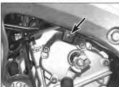
4.19b ... and undo the bolt securing the ABS system pipes
