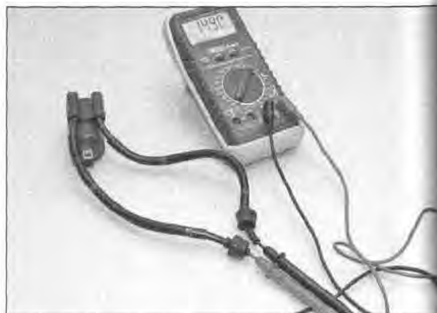
17.5 Checking the coil secondary resistance between the HT leads
