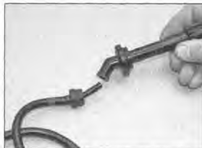
17.3a Unscrew the plug cap from the HT lead ...
