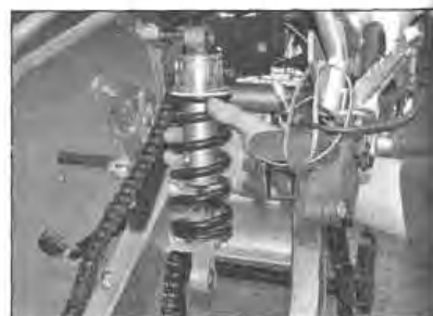
11.6b ... and lift the shock out
