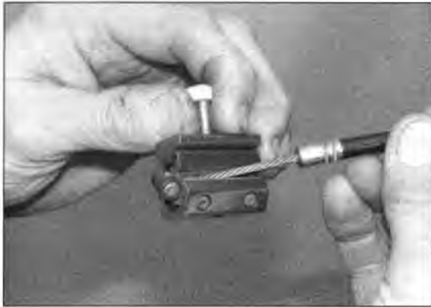
8.5a Fit the cable into the adapter ...
