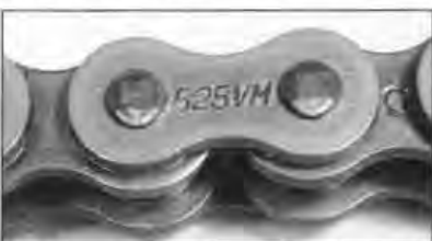
8.10 Typical chain size and type marking
