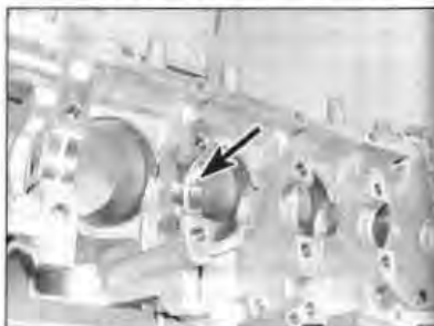
28.9 Inspect the bearing seats and oilways (arrowed)
