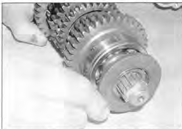
19.10 It is best to fit a new output shaft oil seal before reassembly
