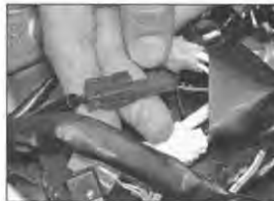
4.3b ... and disconnect its wiring at the 2-pin connector
