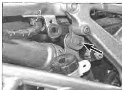
13.4b ... then unscrew the exhaust bracket bolt (arrowed) ...
