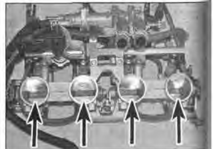
9.19c Check that the butterfly valves (arrowed) close properly against the throttle bodies
