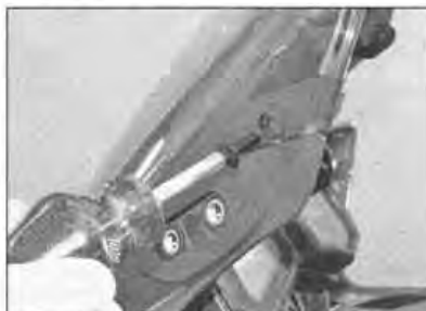
3.2a Undo the screws ...
