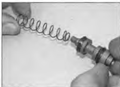
5.15 Fit the narrow end of the spring onto the piston
