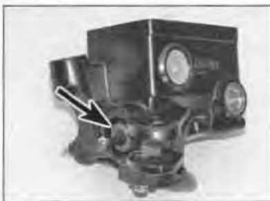
5.17 Ensure the boot is pressed into the recess (arrowed) in the master cylinder
