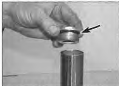
7.2 Note the O-ring (arrowed) on the fork top bolt
