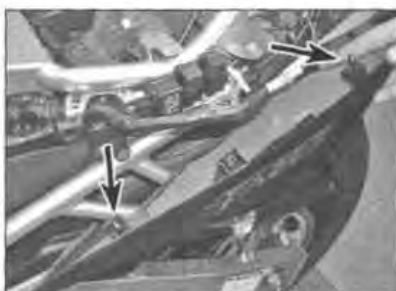
6.3 Note how the pegs (arrowed) locate in grommets
