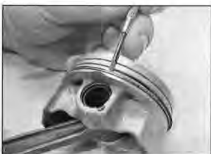
23.8c ... and the upper side rail as described
