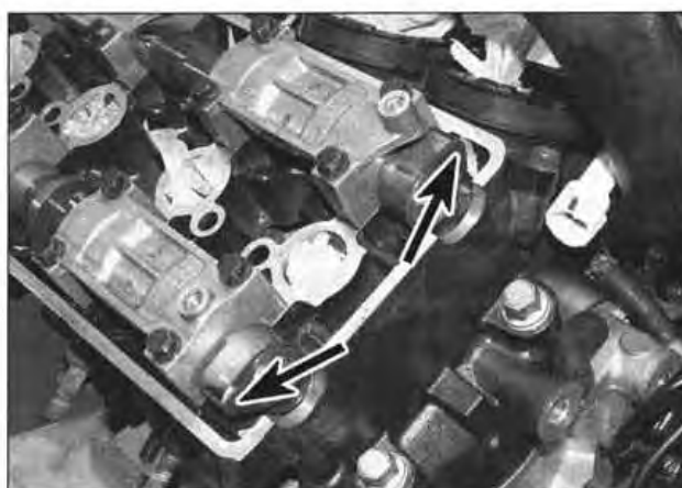
19.8b Ensure the cam lobes (No. 1 cylinder) are facing away from each other as shown
