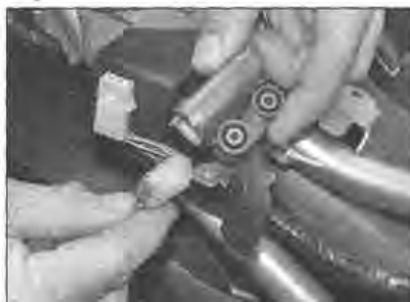
8.43 Note the top surface of the sensor is marked UP
