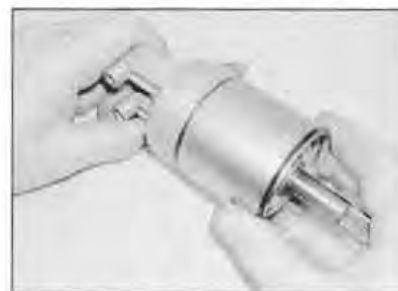
29.5 Carefully draw the main housing off the armature
