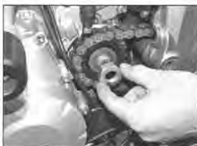
19.12b Undo the sprocket nut ...
