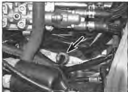
5.4 Location of the coolant temperature sensor (arrowed)
