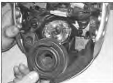
7.2 Note how the cover fits over the back of the headlight reflector
