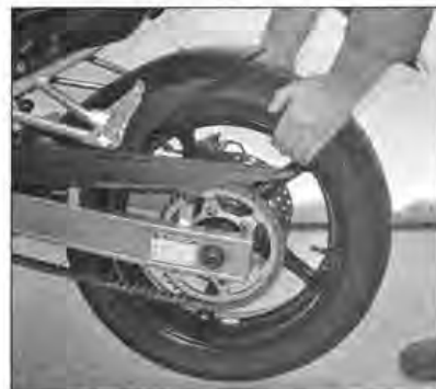
13.9 Checking for play in the rear shock mountings
