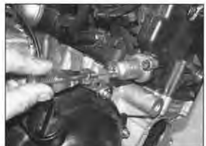
7.4b ... then insert the screwdriver and retract the plunger and unscrew the mounting bolts
