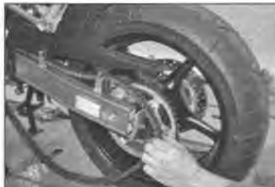
15.6 Disengage the chain from the sprocket
