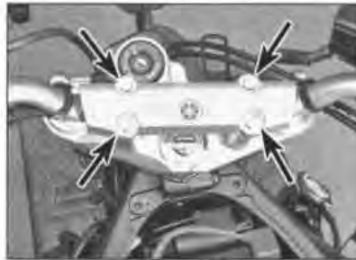
5.11b One-piece handlebar clamp is secured by bolts (arrowed)
