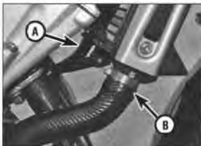
2.6a Detach the oil cooler hose (A), the radiator outlet hose (B) . . .
