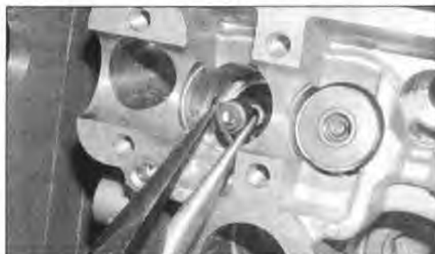
11.9 Pull the stem seal off with long nosed pliers
