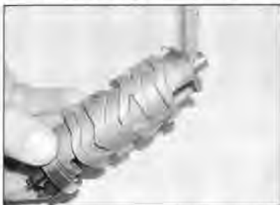
27.16a Lubricate the end of the selector drum before assembly
