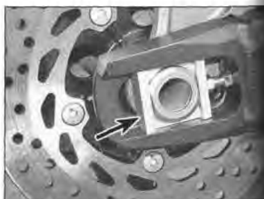
13.14 Chain adjuster plates (arrowed) should be a good sliding fit
