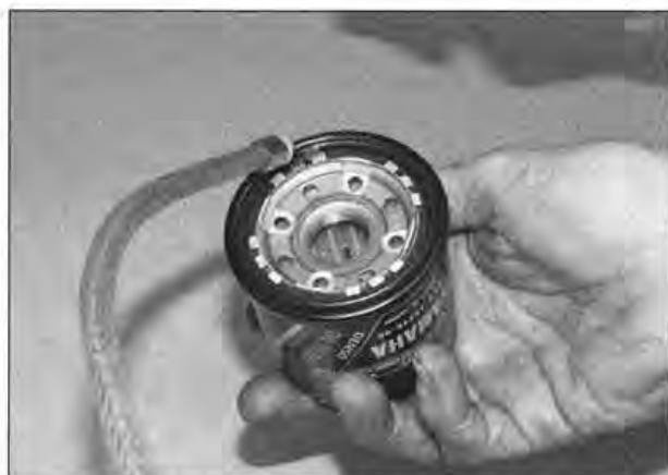
10.11a Lubricate the filter seal with clean oil...
