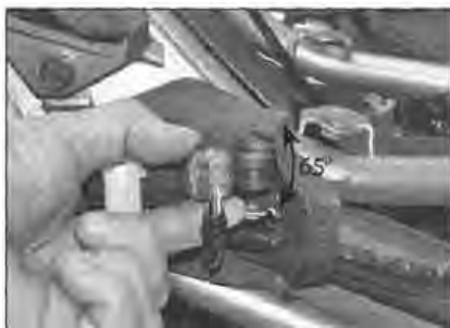
8.41 Tilt the tip-over sensor both ways to check its operation
