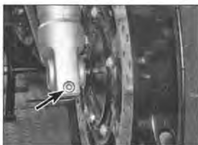
14.3a Slacken the pinch bolt (arrowed) ...
