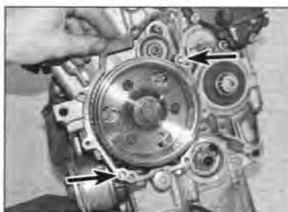
14.16a Fit a new gasket onto the dowels (arrowed) . . .
