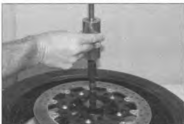
16.4 Using an expanding puller and slide-hammer
