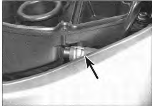
18.7 Location of the AIS hose union (arrowed)
