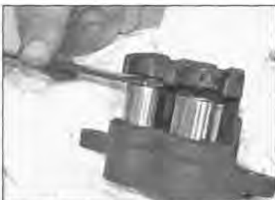
3.7 Blocking one piston while the other is forced out under air pressure
