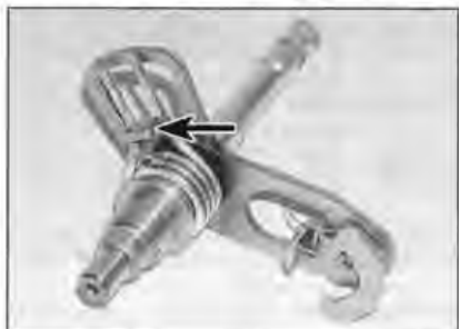
15.14 Centralising spring ends locate on each side of tab (arrowed)
