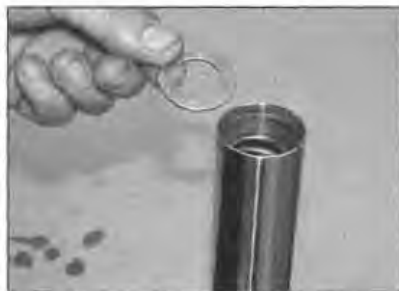
7.3b ... and the washer from the fork leg ...
