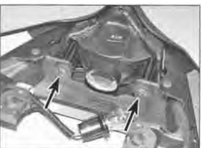
10.3 Tail light unit is secured by two screws (arrowed)
