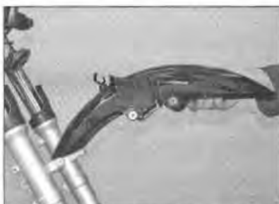
7.9 Draw the mudguard forwards to remove it
