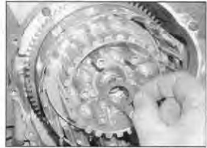
13.36b Align the new lockwasher tabs with the flats on the clutch centre boss
