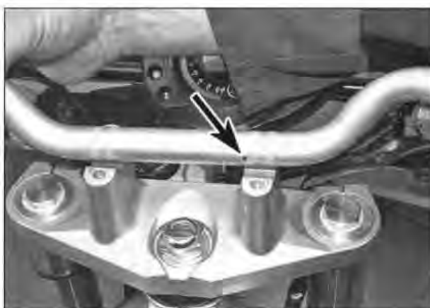
14.15 Align the register mark (arrowed) with the top edge of the lower bracket
