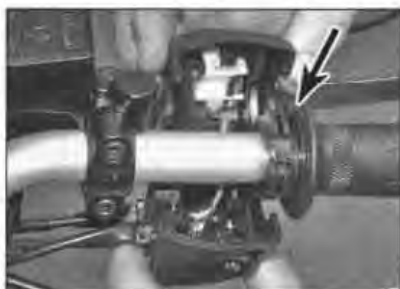
20.3 Removing the right-hand switch unit. Note the throttle twistgrip (arrowed)
