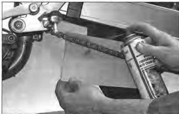
1.18 Protect the rear tyre from overspray when lubricating the chain
