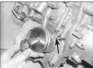
16.4 Remove the oil cooler, noting how the tab (arrowed) locates against the crankcase
