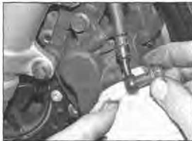
3.3b Detach the banjo fitting, catching any residual brake fluid with rag
