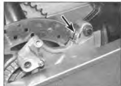
6.5b Location of the pad plate (arrowed)
