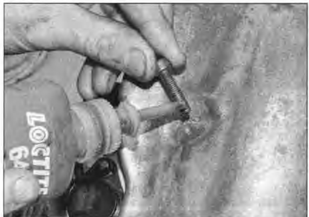
17.12b . . . and apply a thread lock to the central bolt
