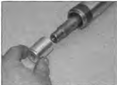
8.19 Fit the damper seat onto the projecting end of the damper
