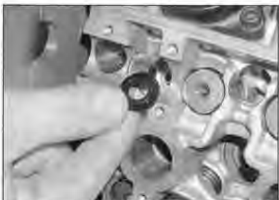
11.29a Install the valve spring seat
