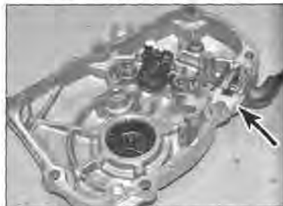
8.10 Apply sealant to the wiring grommet (arrowed)
