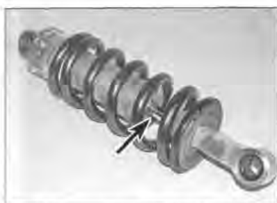
11.8 Check the damper rod for wear, pitting and signs of leakage (arrowed)
