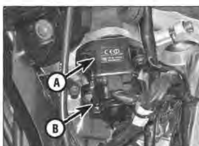
9.7a Location of the immobiliser transceiver (A) and ignition switch (B)
