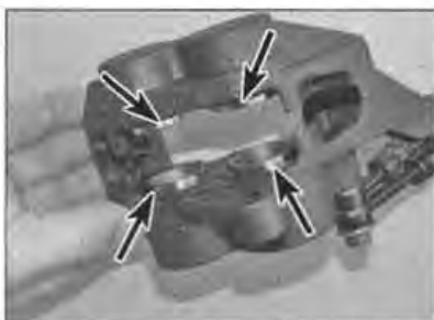
2.25 Ensure the exposed ends of the caliper pistons (arrowed) are clean
