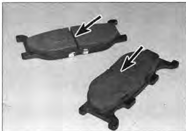
11.14 Note the wear indicator grooves (arrowed)
