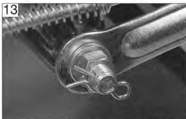
Brake torque arm must be properly secured at both ends
