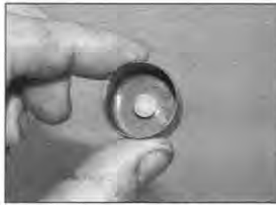
8.13b . . . and retrieve the shim from inside it . . .
