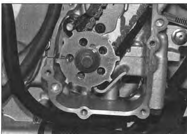
19.8a Align the 'T' mark with the rear facing crankcase mating surfaces
