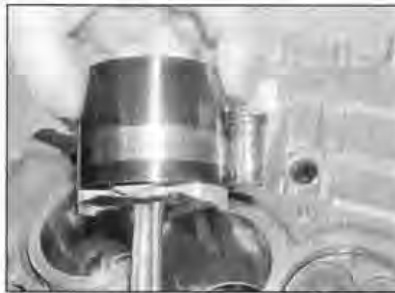
21.32a With the ring ends staggered, fit the ring compressor over the piston ...
