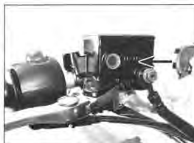
1 The front brake fluid level is visible through a sightglass in the reservoir body – it must be above the LOWER level line (arrowed).
