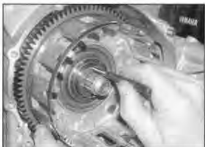
13.16a Use a tool to dislodge the bearing centre from the clutch housing ...
