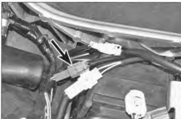
3.14 Location of the rear brake light switch wiring connector (arrowed)
