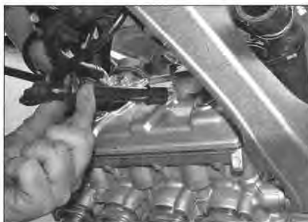
2.3 Pull the caps off the spark plugs
