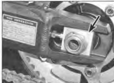
15.4b On S2 models, remove the axle nut, washer and chain adjuster plate (arrowed)
