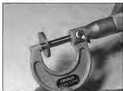
Tappet shims are measured with a micrometer
