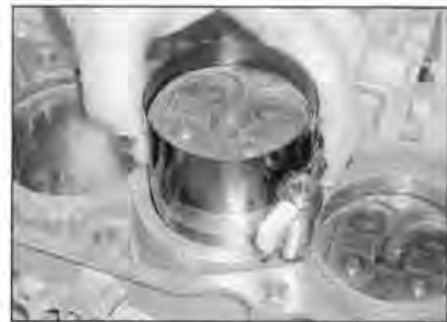
21.32b ... then insert the rod assembly into the top of the bore ...
