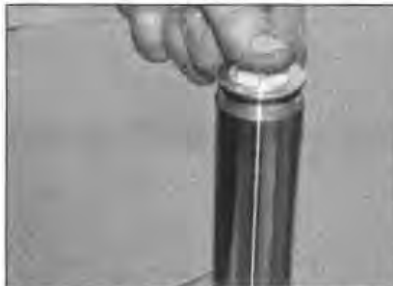
7.9 Press the top bolt down against spring pressure
