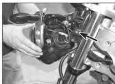
8.2a Note the location of the headlight assembly bracket (arrowed)
