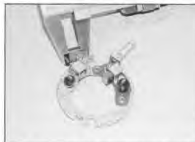
29.10 Measure the length of each brush
