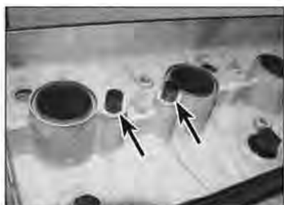
6.4 Take care not to lose the dowels (arrowed)
