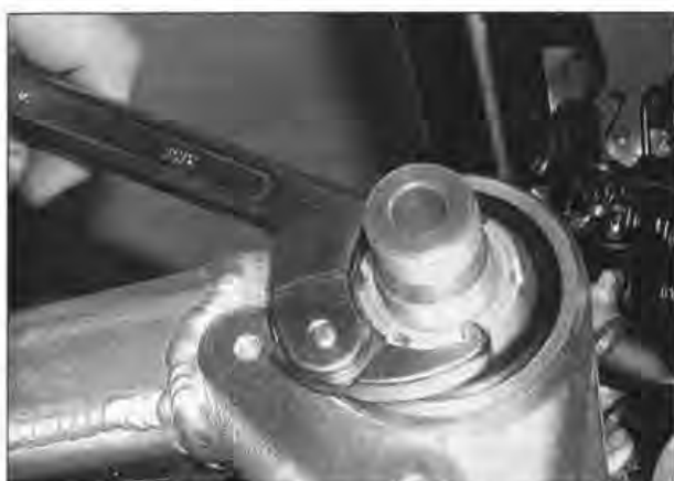
14.11b ... and then tighten the adjuster nut as described to remove bearing freeplay
