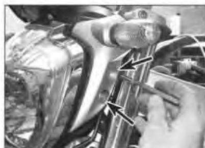
8.1 Headlight assembly is secured by two bolts (arrowed) on each side
