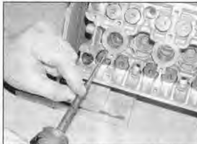
11.33 Tap the valve stem gently to seat the collets in the groove
