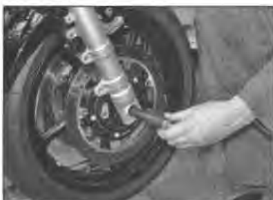
14.4a Unscrew and withdraw the axle
