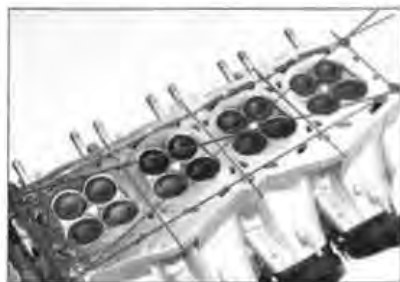
3.23 Check for warpage in these directions
