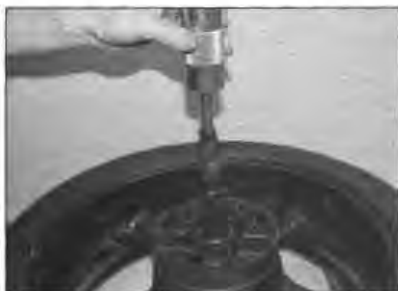
16.15b ... then use the slide-hammer to pull the bearing out
