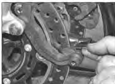
3.19 Fit new pad plates if necessary and ensure they are secure
