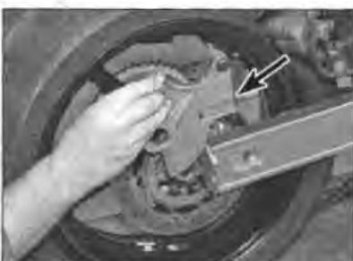
15.15 Locate the slot (arrowed) over the peg on the swingarm
