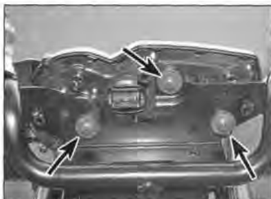
15.8a Instrument cluster on S2 models is secured by three screws (arrowed)
