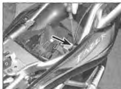
6.2 Location of panel fixing screw (arrowed)
