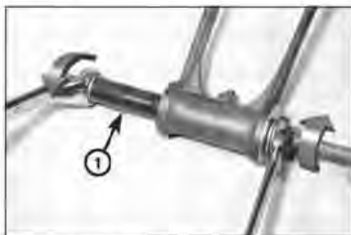
5.11 Installing a new bearing (1) in the suspension arm
