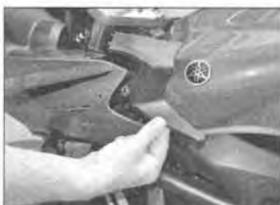
5.1d ... then lift the panel off
