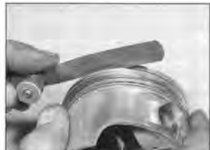
22.11 Measuring the piston ring-to-groove clearance with a feeler gauge
