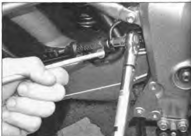
9.22b Tightening the banjo bolt with a torque wrench as described
