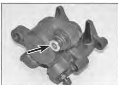
7.17 Location of the slider pin sleeve (arrowed) in the caliper
