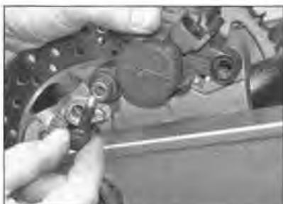
6.19c Hold the caliper down and install the rear slider pin ...
