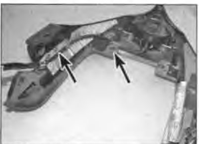
10.2 Note how the wiring sub-loom is secured inside the seat cowl (arrowed)
