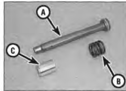
8.16 Examine damper (A), spring (B) and damper seat (C)
