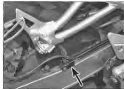
10.4c Brake hose/pipe union located on the swingarm
