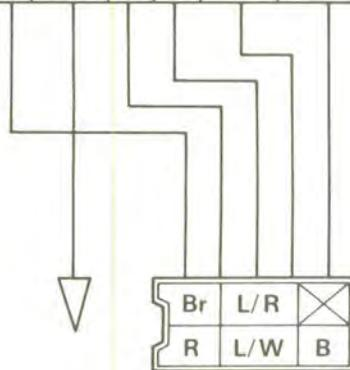
"R and Br" and L/W and L/R" are continuous with the "ON" switch position.
