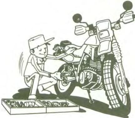
3. When disassembling the motorcycle, keep mated parts together. This includes gears, cylinders, pistons, and other mated parts that have been "mated" through normal wear. Mated parts must be reused as an assembly or replaced.
