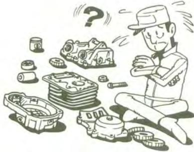
4. During the motorcycle disassembly, clean all parts and place them in trays in the order of disassembly. This will speed up assembly time and help assure that all parts are correctly reinstalled.
