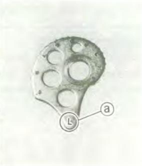
2. Install the chain pullers ① so that the "L" mark ② should be on the left side and the "R" mark on the right side.
