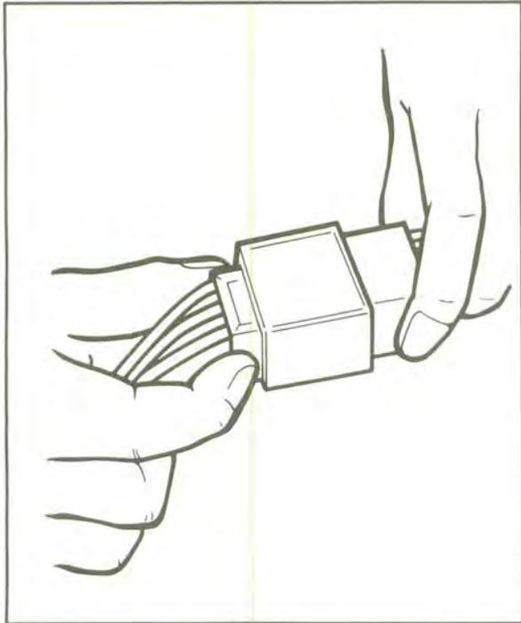
1. Disconnect the main switch coupler from the wire harness.
