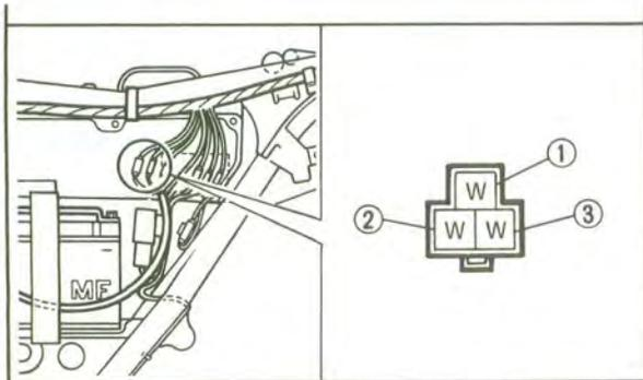
• Check the stator coil for specified resistance.
