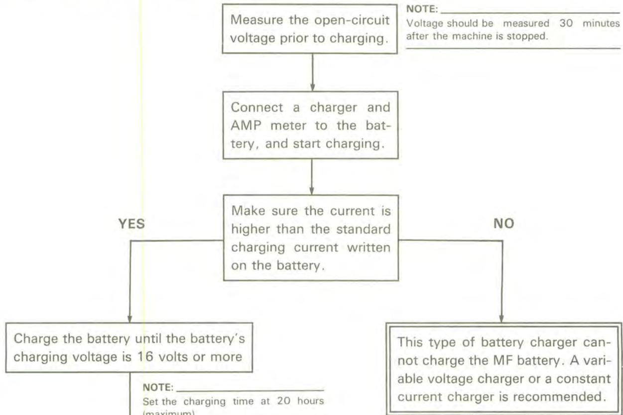
Check the open-circuit voltage after having left the battery for 30 minutes after charging.
