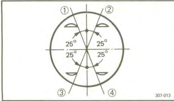
5. Offset the piston ring end gaps as shown.
