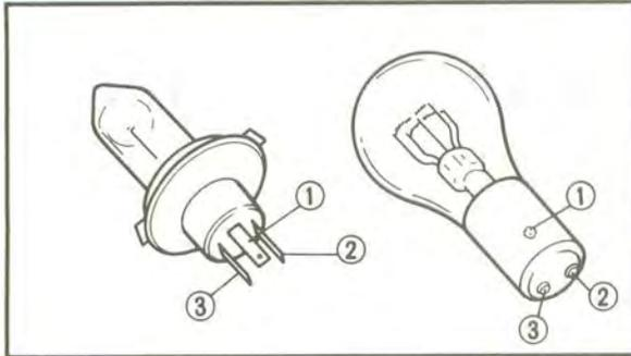
3. Check the bulb socket by installing a proven bulb to it. As in the checking of bulbs, connect the pocket tester leads to the respective leads of the socket and check for continuity in the same manner as mentioned above.
