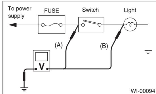
4) With test set-up held as it is, turn the switch ON. The voltmeter will indicate a voltage and, at the same time, the light will come on.
