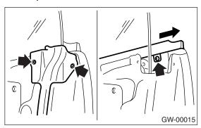
8) Operate the power window switch to move the glass to position shown in the figure, and then remove the two nuts from service holes.
