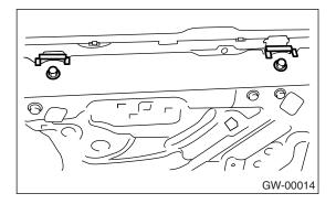
7) Remove the rear end of door weatherstrip and weatherstrip outer.
