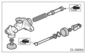
3) To assemble the master cylinder, reverse the sequence of disassembly procedure.
