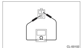
Clutch switch (With cruise control)
