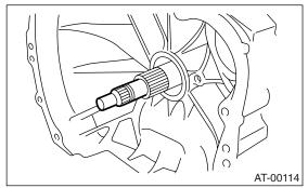
4) Remove the clip from torque converter clutch assembly.
