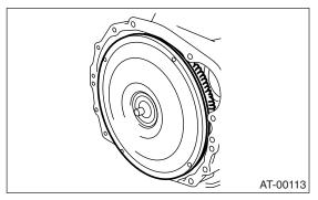
3) Remove the input shaft.
