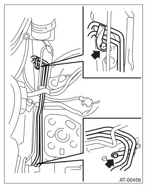
8) Remove the ATF cooler inlet and outlet pipes.
