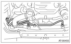
6) Disconnect ATF cooler hoses from pipes.
