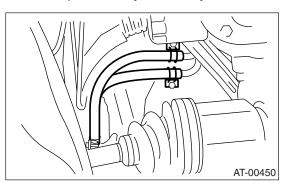
7) Remove ATF cooler pipe from frame.
