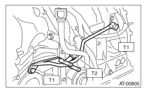
2) Install ATF cooler pipe to frame.
