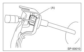
12) Separate the accelerator cable and accelerator bracket.
