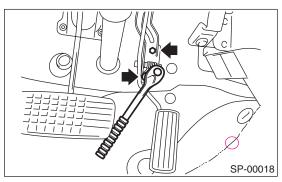
8) Disconnect the grommet from toe board.
