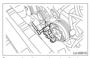
15) Remove the oil pump by using flat tip screwdriver.
