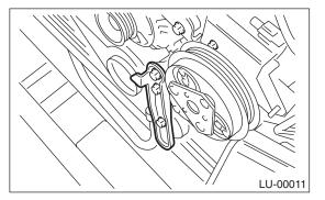
10) Remove the crank pulley by using ST. 499977100 CRANK PULLEY WRENCH
