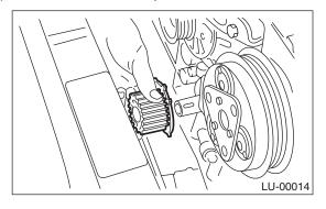
14) Remove the bolts which install oil pump onto cylinder block.
