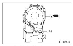
2) Replace the O-ring (A) with a new one.
