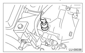
3) Remove the oil pressure switch.
