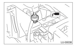
2) Install the oil pressure switch onto engine block.
