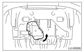
4) Drain the engine oil by loosening the engine oil drain plug.
