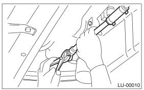
6) Remove the engine oil filter. <Ref. to LU(H4SO)-25, REMOVAL, Engine Oil Filter.> 7) Remove the connector and remove oil cooler.
