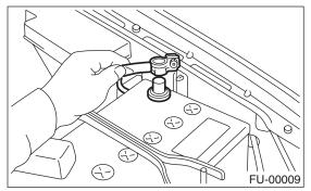
2) Disconnect the connector (A) of intake air temperature sensor.
