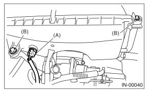
4) Disconnect the hoses and intake duct from air cleaner case.
