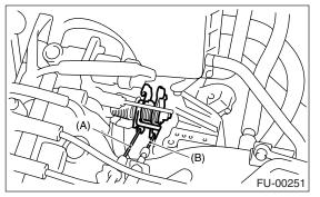
5) Disconnect the connectors from idle air control solenoid valve, throttle position sensor and manifold absolute pressure sensor.
