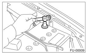
2) Disconnect the connector from the intake air temperature sensor.
