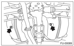
6) Tighten the fuel drain plug.
