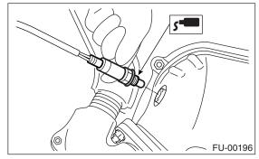
2) Install the front oxygen (A/F) sensor.
