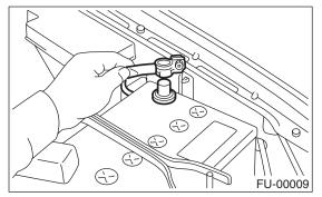
2) Remove the connector from engine hanger, and then disconnect the front oxygen (A/F) sensor connector.
