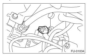
4) Remove the engine coolant temperature sensor.
