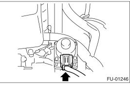
3) Remove the EGR valve from intake manifold.
