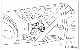
3) Remove the crankshaft position sensor, and disconnect the connector from it.
