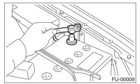
2) Remove the bolt which install crankshaft position sensor to the cylinder block.
