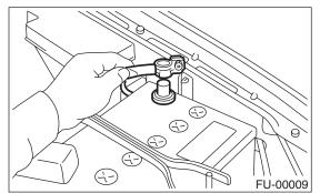
2) Disconnect the connector from the air assist injector solenoid valve and disconnect the air bypass hoses.
