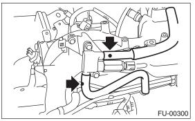
3) Remove the air assist injector solenoid valve from the intake manifold.
