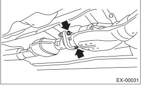
2) Separate the rear exhaust pipe from muffler.
