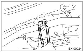
2) Apply a coat of SUBARU CRC to mating area of the cushion rubbers in advance.
