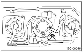
4) Remove the nuts, and then remove the vent valve.
