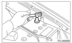
2) Remove the bolt which installs purge control solenoid valve onto intake manifold.
