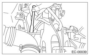
3) Disconnect the connector and hoses from purge control solenoid valve.
