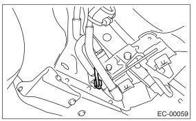
6) Disconnect the evaporation hoses (A) from joint pipes.
