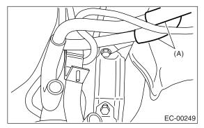
7) Remove the bolt which installs the drain filter and drain valve brackets on body, and remove them as a unit.
