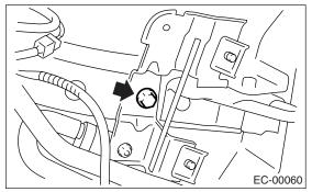
8) Disconnect the evaporation hoses from drain filter.
