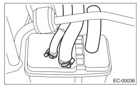
3) Remove the canister from body.
