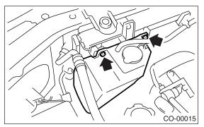
14) Disconnect the radiator inlet hose (A) and water tank hose (B) from radiator.
