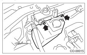
12) Disconnect the radiator inlet hose from radiator.
