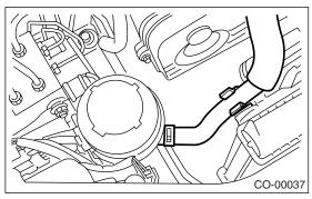
6) Connect the radiator inlet hose (A) and water tank hose (B).
