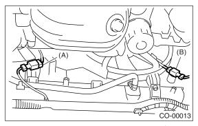
7) Disconnect the radiator outlet hose from water pump.
