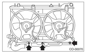
2) Attach the radiator lower cushions to holes on the vehicle.
