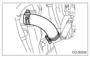
8) Disconnect the ATF cooler hose from ATF pipe. (AT model)
