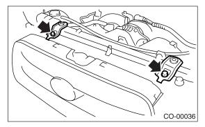
14) Disconnect the power steering hose from clip on radiator.
