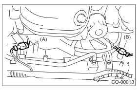
7) Disconnect the radiator outlet hose from thermostat cover.
