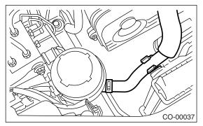
15) Lift the radiator up and away from the vehicle.
