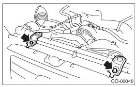
16) Disconnect the power steering hose from clips on radiator.
