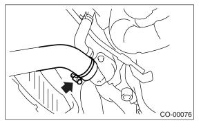
8) Disconnect the ATF cooler hoses from ATF pipe. (AT model)
