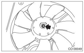
3) Remove the bolts which install fan motor onto shroud.
