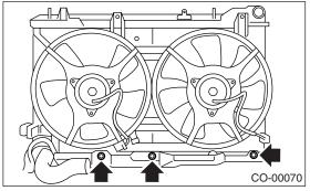
9) Pull the radiator lower hose upward to space radiator from radiator under cover. Remove the ATF hose from two clips on the radiator main fan motor assembly. (AT model)
