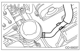
9) Connect the radiator inlet hose to radiator.
