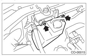
12) Remove the radiator main fan motor assembly mounting bolts.
