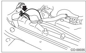
14) Disconnect the power steering hose from clip on radiator.
