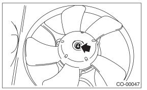
3) Remove the bolts which install fan motor onto shroud.
