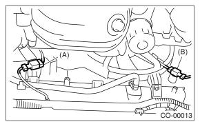
7) Remove the ATF hose from clip of radiator fan motor assembly (AT model).
