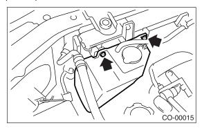
14) Remove the radiator main fan motor assembly securing bolt.
