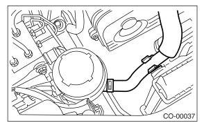
17) Remove the radiator fan motor assembly from vehicle.
