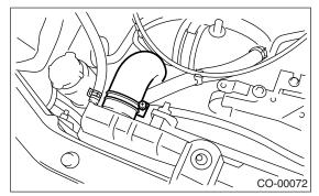
10) Install the radiator main fan motor assembly mounting bolts.
