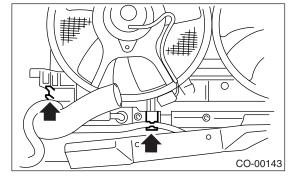
4) Tighten the radiator under cover securing bolt. (AT model)
