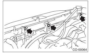
13) Disconnect the radiator inlet hose from radiator.
