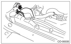
4) Install the radiator main fan motor assembly mounting bolts.
