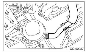
15) Rise up the radiator main fan motor assembly to remove it from vehicle.
