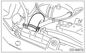
16) Disconnect the power steering hose from radiator clip.
