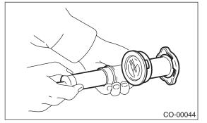
2) Increase the pressure until tester gauge pointer stops. Radiator cap is functioning properly if it holds the service limit pressure for 5 to 6 seconds.
