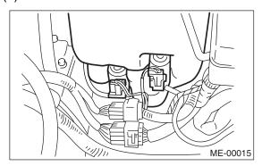
(4) Remove the washer tank mounting bolts.
