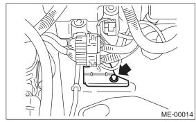
(3) Disconnect the washer motor connectors.
