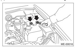
(5) Move the washer tank upward.
