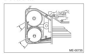
(3) Set the arrow mark on cam sprocket to position shown in the figure, and then measure the #1 cylinder exhaust valve and #4 cylinder intake valve clearances.
