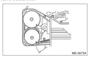
(2) Set the arrow mark on cam sprocket to position shown in the figure, and then measure the #2 cylinder intake valve and #4 cylinder exhaust valve clearances.
