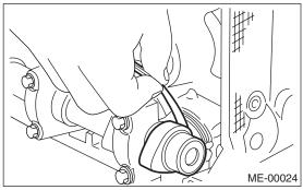
2) Remove the camshaft. <Ref. to ME(H4DOTC)-61, REMOVAL, Camshaft.>
