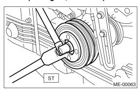
3) Confirm that the tightening angle of crank pulley bolt is 65 degrees or more. If the tightening angle of crank pulley bolt is less than 65 degrees, conduct the following procedures.
