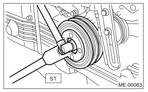
3) Remove the crank pulley.
