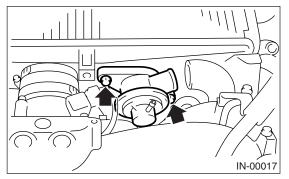
2) Remove the intercooler ducts from intercooler.
