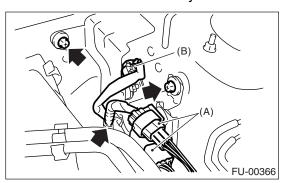
5) Disconnect the pressure hoses (C) from wastegate control solenoid valve.
