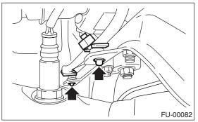
5) Apply SUBARU CRC or its equivalent to the threaded portion of rear oxygen sensor, and leave it for one minute or more.
