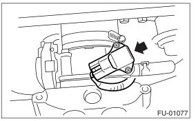
3) Remove the manifold absolute pressure sensor from the throttle body.
