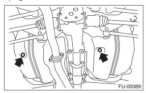
6) Tighten the fuel drain plug.
