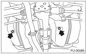
4) Tighten the fuel drain plug.
