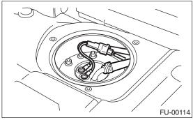
9) Remove the bolts which install the fuel sub meter unit on the fuel tank.
