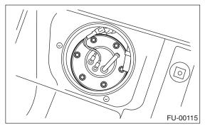
10) Remove the fuel sub meter unit.
