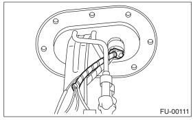
3) Remove the bolt which installs the fuel level sensor on the mounting bracket.
