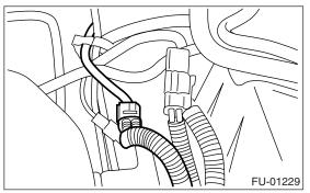
3) Disconnect the engine harness fixed by clip (A) from the bracket (B).
