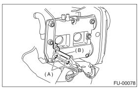
7) Connect the connector of front oxygen (A/F) sensor.
