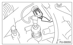
5) Remove the engine coolant temperature sensor.
