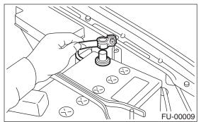
2) Disconnect the exhaust temperature sensor connector.
