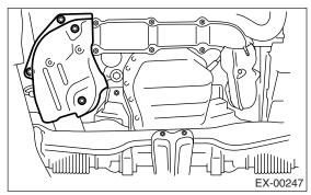
6) Remove the nuts which hold front exhaust manifold to joint pipe.
