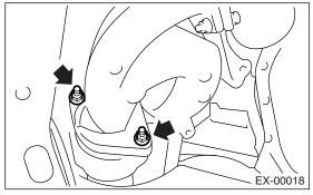
7) Remove the center exhaust pipe. <Ref. to EX(H4DOTC)-8, REMOVAL, Center Exhaust Pipe.>
