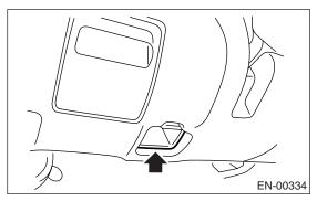
3) Using the OBD-II general scan tool, call up DTC and freeze frame data.
