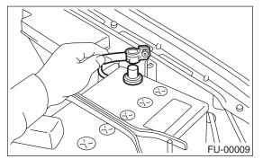
2) Disconnect the connector and hoses from purge control solenoid valve.
