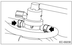
9) Disconnect the vacuum hose from pressure control solenoid valve.
