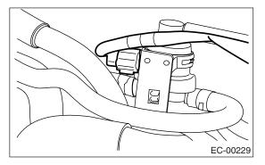
7) Remove the pressure control solenoid valve from bracket.
