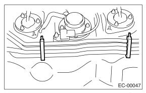
5) Remove the nuts and bolts which install fuel tank pressure sensor on bracket.
