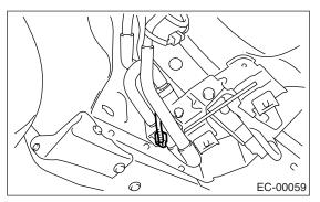
5) Disconnect the evaporation hoses (A) from joint pipes.
