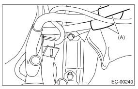
6) Remove the bolt which installs the drain valve and drain valve brackets on body, and remove them as a unit.
