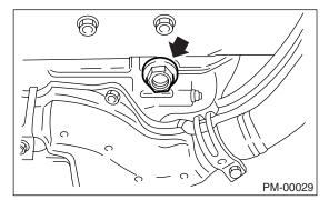
2) Replace the gasket with new one, and then tighten it to the specified torque.
